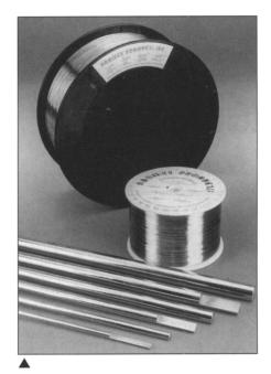
**Nickel-Clad Copper Wire:** Anomet's nickel-clad copper wire features a metallurgical bond with complete hermetic sealing between the metals rather than plating. Available with annealed through full hard tempers, the wire provides 45% IACS conductivity and can be supplied as wire and rod from 0.010-in. to 1-in. in diameter. The standard nickel ratio is 27%, with 10 to 40% Ni optional.
