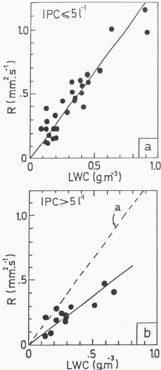
Fig.1. Icing rate  $R$  plotted against cloud liquid water content  $LWC$ :
