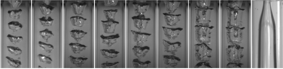
FIGURE 12. Transition from bubbly flow to annular flow inside a drainpipe.
