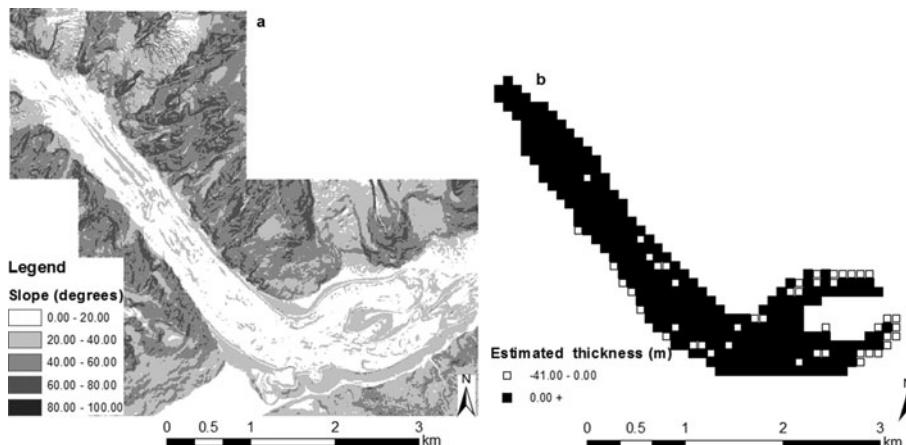
**Fig. 9.** (a) Slope map derived from 2008 lidar DEM (2 m resolution) and (b) plot showing location of negative debris-thickness estimates ( $d$ ) from SLOPEMOD in 2005 ( $z_0 = 0.016$  m), which were subsequently set to the values obtained at corresponding pixels using FLATMOD.
