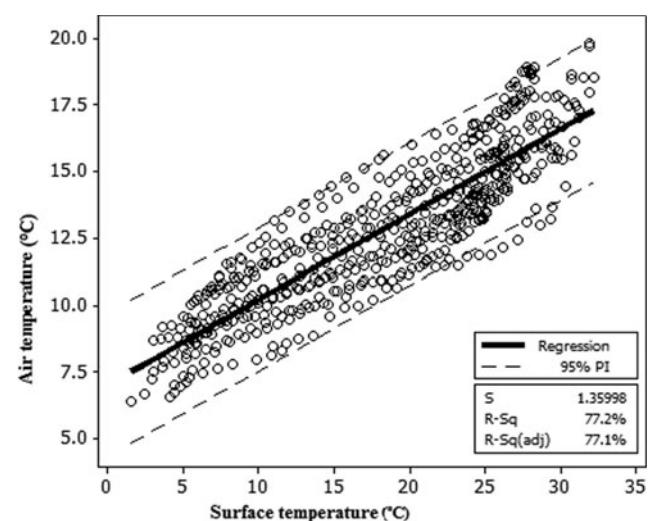
**Fig. 6.** Relationship of 2 m air temperature to debris surface (radiative) temperature under clear-sky conditions between 08:00 and 14:00 recorded at the AWS during the 2005 season. The outer dashed lines are the 95% prediction intervals; 575 data points; 10 min average values. Data for days with wind speed  $>5.9\text{ m s}^{-1}$  not included.
