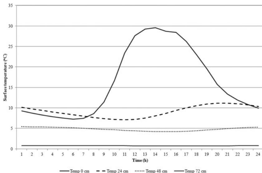
**Fig. 4.** 2005 average daily temperature cycles over a 10 day period of fine weather (21–30 July 2005) at four levels in a 0.72 m debris layer. The values show depth below the surface, and 0.72 m is at the debris–ice interface.
