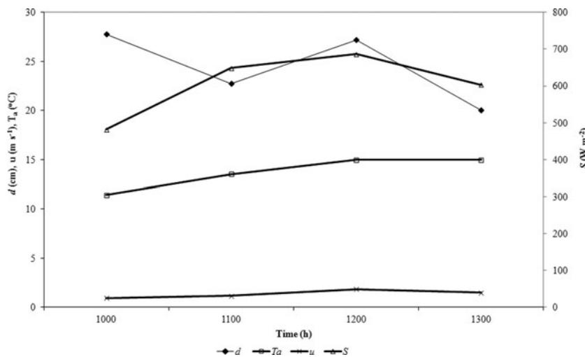
**Fig. 5.** Modelled debris thickness,  $d$ , at the AWS site on 1 August 2005 between 10:00 and 13:00 using measured input variables and  $z_0=0.006\text{ m}$ .  $d$  is the estimated debris thickness (cm),  $T_a$  is the air temperature at 2 m ( $^{\circ}\text{C}$ ),  $u$  is wind speed at 2 m ( $\text{m s}^{-1}$ ) and  $S$  is the net shortwave radiation flux ( $\text{W m}^{-2}$ ).
