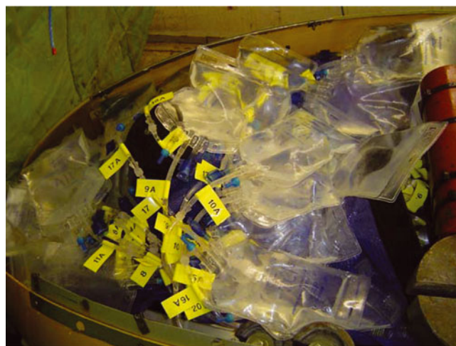
Fig. 4. The AquaLab water sampler located in the nose of the Autosub vehicle. Individual water-sample bags are visible. Photograph by P. Dodd.
