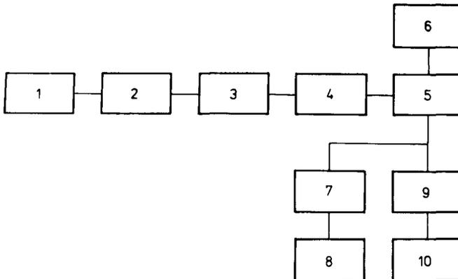
Figure 1. Block schematic of the TV spectrometer: 1, Telescope; 2, Grating spectrometer; 3, TV system; 4, 7, 9, Interfaces; 5, Computer (15 BSM-5); 6, Magnetic tape; 8, Teletype; 10, Perforator.
