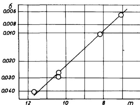
Figure 8. The mean square error of one intensity ratio measurement in the continuum as a function of stellar magnitude.
