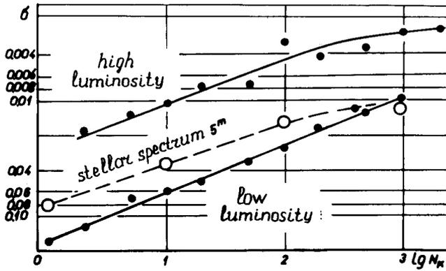
Figure 3. Mean square error of measured intensity per channel shown as a function of the number of integrated readouts. The solid curves are from laboratory measurements. The dashed curve is from the measurement of a 5<sup>m</sup> AO star using a 0.5m telescope.
