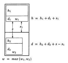
Fig. 4. Two nodes placed above each other.
