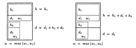
Fig. 3. Two examples for vertical combinations.
