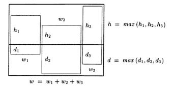
Fig. 2. A horizontal combination of three boxes.
