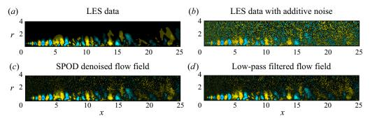
Figure 10. Comparison of noisy and denoised instantaneous pressure fields: (*a*) original LES data; (*b*) LES data with additive Gaussian white noise; (*c*) SPOD-based denoised flow field; (*d*) low-pass filtered flow field. Denoising is achieved by rejecting all SPOD eigenpairs with  $\lambda < 5 \times 10^{-5}$ . This hard threshold is indicated in figure 9.
