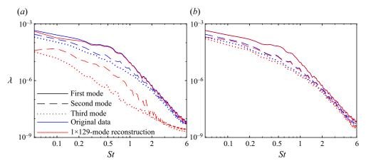
Figure 7. Comparison between SPOD eigenvalue spectra of the original data (blue lines) and  $1 \times 129$ -mode reconstructions (red lines): (a) frequency domain; (b) time domain. Solid, dashed and dotted lines denote the first, second and third modes, respectively.
