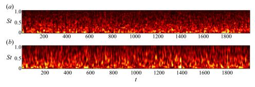
Figure 12. The SPOD-based frequency–time diagrams obtained using the time-domain approach: (*a*) first ten modes at each frequency; (*b*) leading mode at each frequency. The SPOD of the pressure field is considered.
