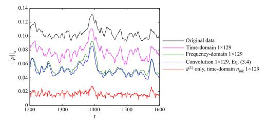
Figure 14. Temporal evolution of the pressure 2-norm in the vicinity of its global maximum at t = 1380. The convolution approach, based on (3.4), is compared to the time- and frequency-domain approaches, previously shown in figure 4(*b*,*d*). The 1 × 129-mode reconstructions are shown.
