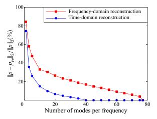
Figure 8. The 2-norm error of the pressure field reconstructed with different rank approximation: (red lines with squares) reconstruction in the frequency domain; (blue lines with circles) reconstruction in the time domain.
