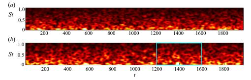
Figure 13. The SPOD-based frequency-time diagrams obtained using the convolution approach: (a) first ten modes at each frequency; (b) leading mode at each frequency. The SPOD of the pressure field is considered. The cyan box in (b) is centred around the global maximum of the instantaneous energy at t = 1380, analysed in figures 14 and 15(c,d) below.
