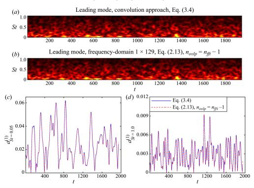
Figure 24. Comparison between two strategies for SPOD-based frequency-time analysis: frequency-time diagrams for (*a*) the convolution approach (SPOD modes precomputed with 50%, overlap) and (*b*) the frequency-domain approach using  $n_{ovlp} = n_{fft} - 1$ ; expansion coefficients for (*c*) St = 0.05 and (*d*) St = 1.0.
