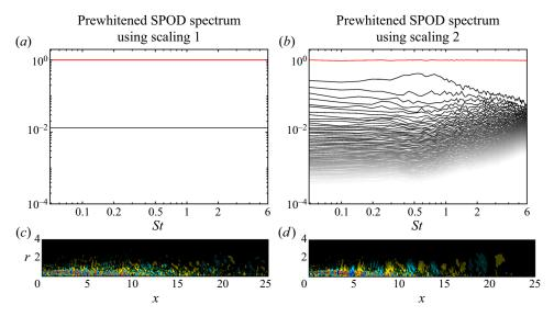
Figure 18. The SPOD-based prewhitening: (a,b) rescaled SPOD spectra; (c,d), instantaneous pressure fields using definitions (3.7) and (3.8), respectively. Red lines indicate the sum of all eigenvalues, that is, the integrated PSD. All lines in (a) collapse owing to the scaling. The original SPOD eigenvalue spectrum can be seen in figure 2(a).
