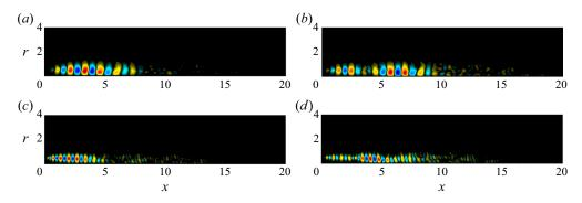
Figure 3. The SPOD modes at St = 0.5 (*a*,*b*) and at St = 1.0 (*c*,*d*). The leading modes are shown in (*a*,*c*) and the suboptimal modes are shown in (*b*,*d*). (*a*) SPOD mode 1, St = 0.50, (*b*) SPOD mode 2, St = 0.50, (*c*) SPOD mode 1, St = 1.00 and (*d*) SPOD mode 2, St = 1.00.
