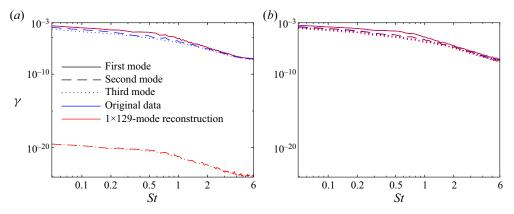
Figure 21. Comparison between SPOD eigenvalue spectra of the original data (blue lines) and  $1 \times 129$ -mode reconstructions (red lines): (*a*) frequency domain; (*b*) time domain. Solid, dashed and dotted lines denote the first, second and third modes, respectively. This figure is identical to figure 7, but for a rectangular window and no overlap.
