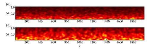
Figure 23. The SPOD-based frequency–time diagrams obtained using the moving mean of the time-domain oblique projection based approach: (*a*) first 10 modes at each frequency; (*b*) leading mode at each frequency. The moving mean uses as weights the same Hamming windowing function as the SPOD.
