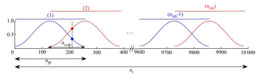
Figure 1. Schematic representation of overlapping blocks, Hamming window and the SPOD parameters such as  $n_t$ ,  $n_{fft}$ ,  $n_{ovlp}$  and  $n_{blk}$ . The left and right blocks are denoted using blue and red lines, respectively. The vertical line corresponds to the snapshot number 210, and the blue and red circles indicate the corresponding value of the window function.
