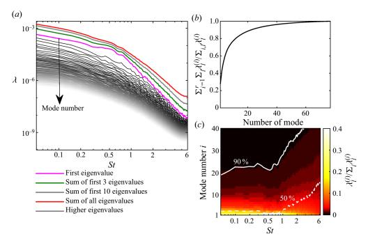
Figure 2. The SPOD spectra of the turbulent jet for m = 1. All eigenvalues (grey lines) and the sum of all eigenvalues (red line), corresponding to the integral PSD, are shown. The normalised cumulative energy content and the percentage of energy accounted by each mode as a function of frequency are shown in (*b,c*), respectively. The solid and dashed white lines indicate the number of modes required to retain 90 % and 50 % energy at each frequency.
