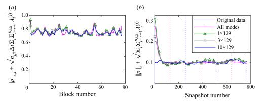
Figure 5. Low dimensional reconstruction in the frequency-domain with truncation correction: (*a*) space–time norm; (*b*) spatial norm. Panels (*a*,*b*) correspond to figure 4(a,b), respectively, but with a correction for the truncated modes. The correction is facilitated by adding the energies of the truncated modes (given by their SPOD eigenvalues).
