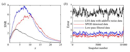
Figure 11. Comparison of the two denoising strategies: (*a*) the SNR along the lipline (r = 0.5) for the noise added flow field (black line), SPOD-based denoised flow field (red lines), and the low-pass filtered flow field (blue line); (*b*) error of the noisy data, SPOD-based denoised data, and the low-pass filtered data. The amplitude of the additive noise was adjusted such that the average SNR along the lipline is one.
