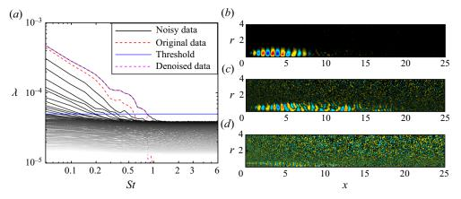
Figure 9. The SPOD of data subjected to additive Gaussian white noise: (a) SPOD spectrum (black lines), leading SPOD eigenvalue of the original data (red dashed line), threshold of  $5 \times 10^{-5}$  (blue line) and the leading SPOD eigenvalue of the denoised data (magenta dashed line); (b) leading SPOD mode at St = 0.5; (c) fifth SPOD mode at St = 0.5; (d) leading SPOD mode at St = 1.5.
