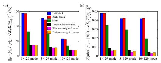
Figure 19. Errors of different ways to compute the frequency-domain reconstruction for  $1 \times 129$ ,  $3 \times 129$  and  $10 \times 129$  modes: (a) 2-norm; (b) spatial norm (2.2). Analogous to figure 5, the residual energy of the truncated modes is subtracted for comparison.
