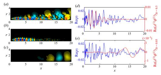
Figure 17. Contributions of individual modes to the reconstructed flow field: (*a*) instantaneous pressure field; (*b*) contribution of  $\phi^{(1)}$  for St = 0.5 and (*c*) for St = 0.05; (*d*) and (*e*) comparisons of the real part of the pressure field along the lipline (r = 0.5) for St = 0.5 and St = 0.05, respectively. The instantaneous flow field at t = 1150 (see figure 15) is shown. Contours in (*a*–*c*) are reported on the same colour axis.
