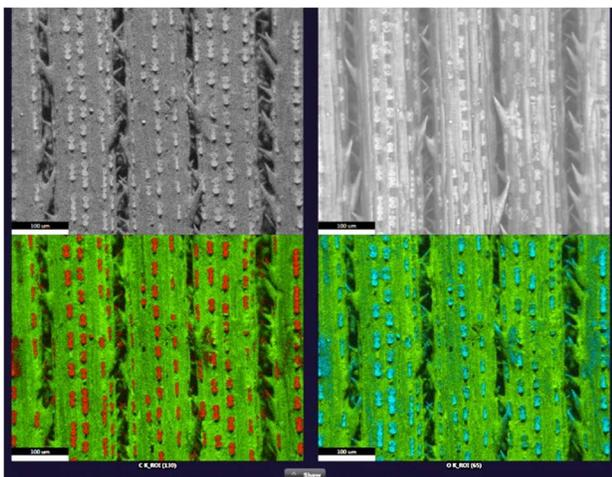
**Figure 1.** SEM image and EDS maps showing Silicon and Oxygen which are present below the surface of a blade of sawgrass [2].
