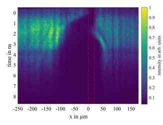
**Figure 8.** Streaked shadowgraphy of a 20  $\mu$ m thick gold target located at  $x = 0 \mu$ m. The initial position is indicated by the red dashed lines. The laser hits the target at t = 0 from the left-hand side, leading to an expansion of the plasma, which is monitored for a duration of almost 10 ns.
