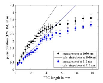
**Figure 4.** Dependency of the pulse duration at 1030 nm (black) and 515 nm (blue) on the length of the FPC used for the seed generation. The black and blue lines correspond to the calculated pulse duration at central wavelengths of 1030 and 515 nm, respectively, given by the cavity ring-down using a reflectivity of 99.7% for both mirrors.
