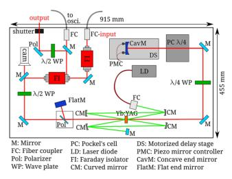
Figure 3. Schematic drawing of the regenerative amplifier with a total size of 915 mm  $\times$  455 mm. The input pulse enters the amplifier through a fiber coupler (red input), passes two Faraday isolators and enters the main cavity, delimited by the flat and concave mirrors (blue). The cavity is set up around a Yb:YAG crystal, which is being pumped by a 12-pass pump system, powered by a laser diode.
