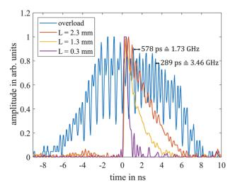
**Figure 5.** Shape of the pulse duration using FPC distances of 0.3 mm (purple), 1.3 mm (yellow) and 2.3 mm, as well as the resulting pulse using the overload (OL) mode of the amplification cavity (blue).
