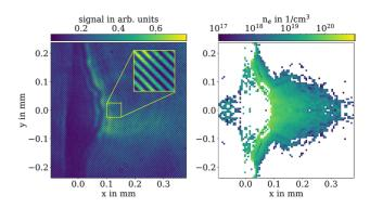
Figure 9. The left-hand side shows an interferometric measurement of a plasma expansion, and the inlet shows a zoomed region of the resulting interference fringes. The right-hand side shows the electron density distribution, extracted from the plasma refractive index of the left-hand side measurement.
