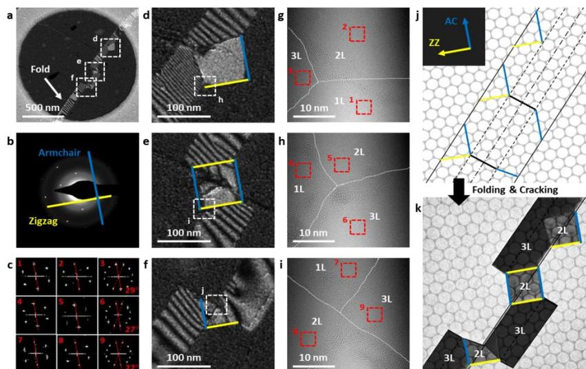
**Figure 1.** (a) DF TEM image showing graphene fold in monolayer graphene. (b) SAED pattern obtained from the whole region in (a). (d-f) Magnified Dark-field TEM images of the regions marked in (a). (g-i) AR TEM images showing graphene fold regions marked in (d-f). (c) FFT patterns obtained from the regions marked in (g-i). (j-k) A paper kirigami illustrating the structure of graphene fold in (a).
