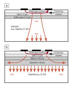
Figure 1. (a) Standard GaN-on-silicon substrate, and (b) GaN-on-silicon-on-diamond (SOD) substrate.
