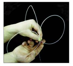
Figure 1. Illustration of a shape-sensing technology that tracks the position of a cable to a high degree of accuracy along its entire length. The shape/position measurement is direct; it does not need to be inferred from other parameters and is completely independent.
