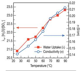
Figure 1. Water uptake and proton conductivity results for a water-retaining polymer electrolyte membrane as a function of temperature at fixed ion contents at RH = 98%.  $\lambda_w$  is the number of water molecules per sulfonic acid group; % water uptake = (mass of water in membrane/mass of dry membrane) × 100.
