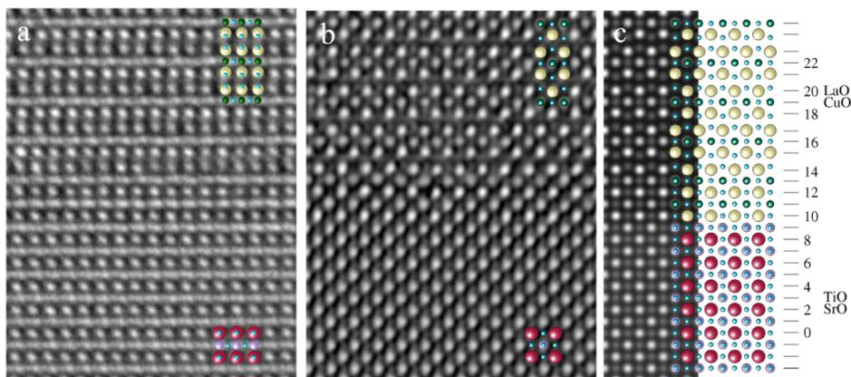
Fig. 1: Atomic structure of the La214/STO interface. (a) NCSI image taken along the [110] viewing direction. (b) Phase of the exit-plane wavefunction reconstructed from a focal series taken in the [100] zone axis. (c) Structure model superimposing the phase of the simulated exit-plane wavefunction along the [100] viewing direction.
