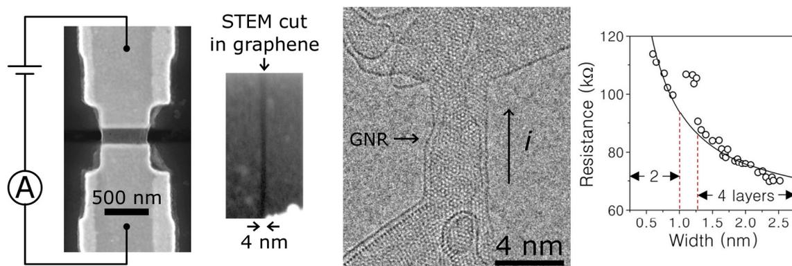
**Figure 2.** From left to right: SEM image of a GNR with electrical contacts, HAADF STEM image showing a straight cut made in STEM mode, HRTEM of a GNR, and GNR resistance as a function of width from data extracted from *in-situ* S/TEM experiments.
