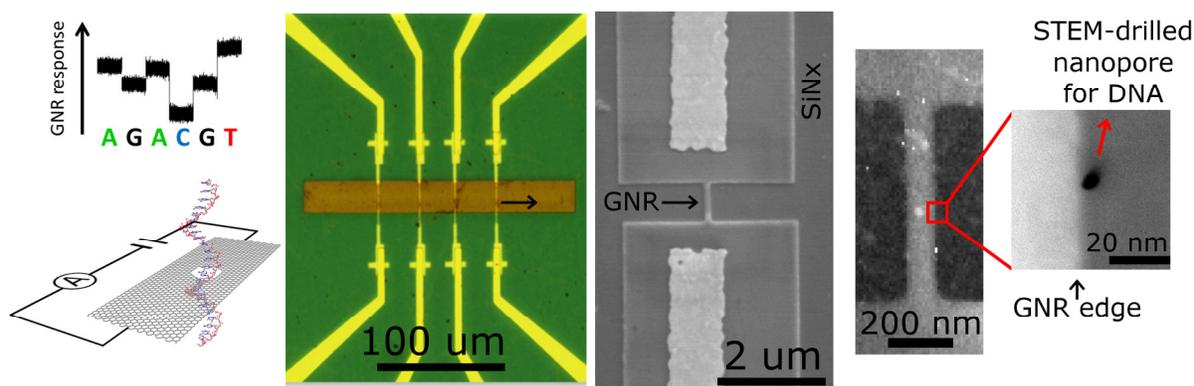
**Figure 1.** From left to right: scheme of GNR-nanopore device for DNA sequencing, optical image of TEM-compatible chip with 4 GNR-nanopore devices, SEM image of a GNR without a nanopore, and STEM image of a GNR-nanopore device.
