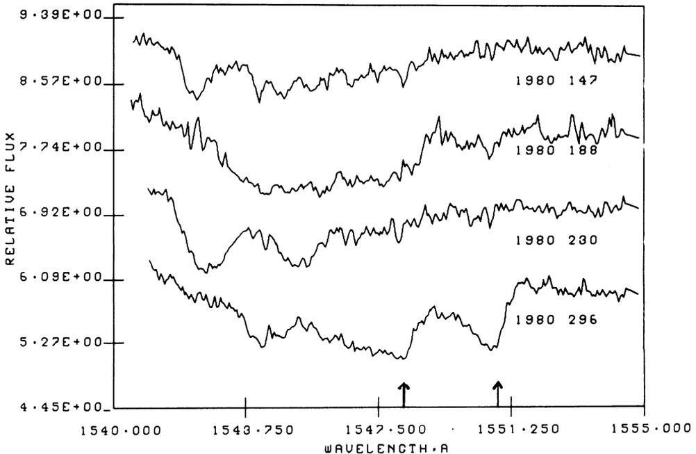
Fig. 1. Representative profiles of CIV resonance lines of 59 Cyg in 1980 ; the arrows show laboratory wavelengths.
