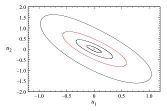
Figure 6. Phase diagram giving the periodic orbits for values of A (7060, 7100, 7200, 7500) close above the oscillatory instability threshold ( $A_c = 7051.36$ , red open circle) for a pure streaming flow (Ra = 0, 2-D cavity with  $A_y = 10$ ,  $H_b = 0.338$ , Pr = 1). Here,  $u_1$  and  $u_2$  are the vertical velocities at the points (x = 0.16055, y = 0) and (x = 0.05437, y = 0.46822), respectively. The cycle presented in figure 7 is given in red.
