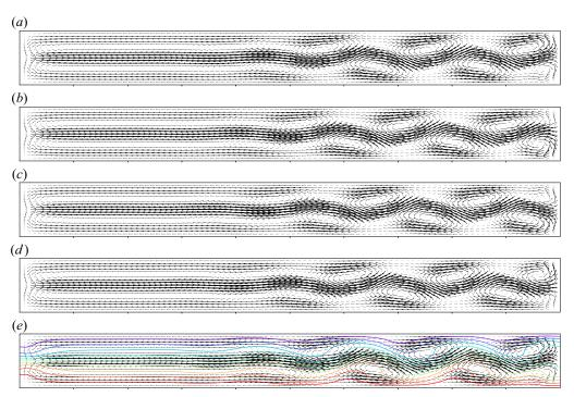
Figure 16. Velocity vectors plots during a cycle at A=4000 and for Ra=6800 (the oscillatory instability threshold is at  $Ra_c=6609.92$  and corresponds to the instability  $I_1$ , see table 3). The period of this cycle is  $T_{osc}=0.4419$  and 5 plots are given, each  $T_{osc}/4$  from 0 to  $T_{osc}$ . For  $t=T_{osc}$  (last plot e), the isotherms are also given (2-D cavity with  $A_y=10$ ,  $H_b=0.338$ , Pr=1).
