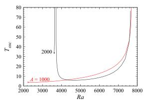
Figure 26. Variation of the period beyond the oscillatory instability thresholds (given as open circles) for two values of the acoustic streaming parameter, A = 1000 and 2000 (2-D cavity with  $A_y = 10$ ,  $H_b = 0.338$ , Pr = 1).
