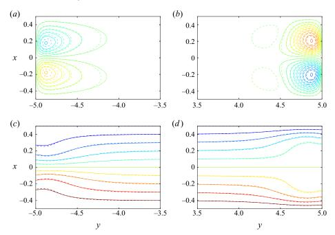
Figure 4. Vertical velocity (a,b) and isotherm (c,d) contours plots in the cavity for A=4000 at the threshold  $Ra_c$  (dashed lines, see text in § 5 and table 3 for details) and at Ra=0 (solid lines, pure streaming). Zooms on the end parts of the cavity (2-D cavity with  $A_v=10$ ,  $H_b=0.338$ , Pr=1).
