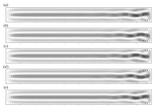
Figure 19. Velocity vectors plots during a cycle at A = 6000 and for Ra = 5400 (the oscillatory instability threshold is at  $Ra_c = 5134.74$  and corresponds to the instability  $I_3$ , see table 3). The period of this cycle is  $T_{osc} = 0.28639$  and 5 plots are given, each  $T_{osc}/4$  from 0 to  $T_{osc}$  (2-D cavity with  $A_y = 10$ ,  $H_b = 0.338$ , Pr = 1).
