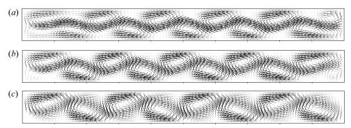
Figure 30. Velocity vectors plots for the stable steady flows obtained for A = 2320 at Ra = 4700 (a), 6000 (b) and  $10\,000$  (c). These stable solutions belong to the loci presented in figure 29(a), as well as the stable solutions obtained by up–down symmetry from these ones (2-D cavity with  $A_v = 10$ ,  $H_b = 0.338$ , Pr = 1).
