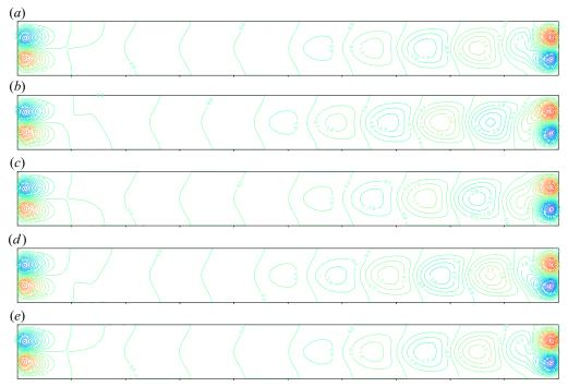
Figure 22. Vertical velocity contour plots during a cycle at A = 2000 and for Ra = 3630 (the oscillatory instability threshold is at  $Ra_c = 3621.62$ , see table 3). The period of this cycle is  $T_{osc} = 41.711$  and 5 plots are given, each  $T_{osc}/4$  from 0 to  $T_{osc}$  (2-D cavity with  $A_y = 10$ ,  $H_b = 0.338$ , Pr = 1).
