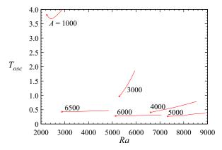
Figure 15. Variation of the period beyond the oscillatory instability threshold (given as a red open circle) for different values of the acoustic streaming parameter A. The characteristics at the critical thresholds, type of instability, critical Rayleigh number  $Ra_c$  and critical period  $T_{osc,c}$  are given in table 3 (2-D cavity with  $A_y = 10$ ,  $H_b = 0.338$ , Pr = 1).
