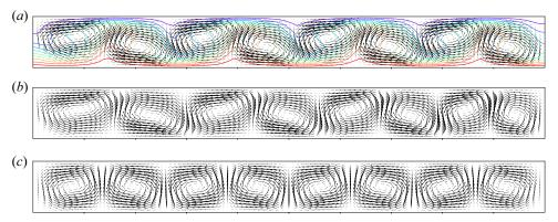
Figure 32. Velocity vector plots for the stable steady flows initiated at the upper saddle-nodes curve  $SN_{U_2}$  in figure 20 for A=2000 and Ra=9000 (a), A=1000 and Ra=9000 (b), A=0 and Ra=4000 (c). For A=2000 (a), the isotherms are also given. The steady flows obtained by up–down symmetry from these ones are also stable solutions (2-D cavity with  $A_y=10$ ,  $H_b=0.338$ , Pr=1).
