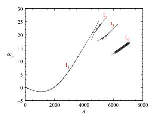
Figure 9. Critical angular frequency at the onset of instability in the Rayleigh–Bénard–Eckart problem in a long 2-D cavity expressed as  $\omega_c$  as a function of A ( $A_y = 10$ ,  $H_b = 0.338$ , Pr = 1).
