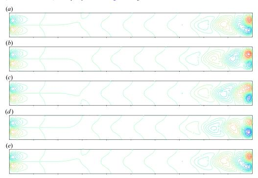
Figure 18. Vertical velocity contour plots during a cycle at A = 5000 and for Ra = 7500 (the oscillatory instability threshold is at  $Ra_c = 7334.14$  and corresponds to the instability  $I_2$ , see table 3). The period of this cycle is  $T_{osc} = 0.27645$  and 5 plots are given, each  $T_{osc}/4$  from 0 to  $T_{osc}$  (2-D cavity with  $A_y = 10$ ,  $H_b = 0.338$ , Pr = 1).
