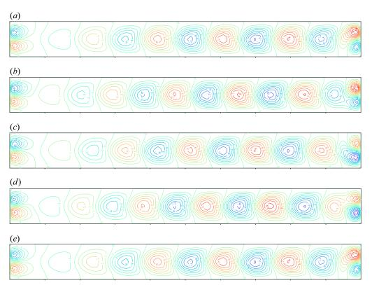
Figure 24. Vertical velocity contour plots during a cycle at A = 2000 and for Ra = 3800 (the oscillatory instability threshold is at  $Ra_c = 3621.62$ , see table 3). The period of this cycle is  $T_{osc} = 15.233$  and 5 plots are given, each  $T_{osc}/4$  from 0 to  $T_{osc}$  (2-D cavity with  $A_v = 10$ ,  $H_b = 0.338$ , Pr = 1).
