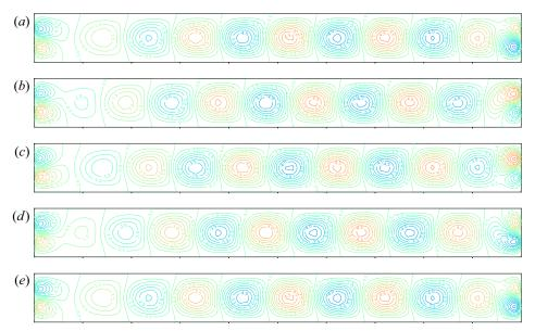
Figure 13. Vertical velocity contour plots during a cycle at A = 1000 and for Ra = 2400 (the oscillatory instability threshold is at  $Ra_c = 2246.97$  and corresponds to the instability  $I_1$ , see table 3). The period of this cycle is  $T_{osc} = 3.6790$  and 5 plots are given, each  $T_{osc}/4$  from 0 to  $T_{osc}$  (2-D cavity with  $A_y = 10$ ,  $H_b = 0.338$ , Pr = 1).
