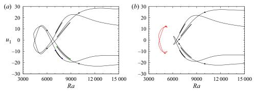
Figure 29. Loci in the parameter space for the steady solutions at A = 2320 (a) and A = 2280 (b) in a 2-D cavity with aspect ratio  $A_y = 10$  ( $H_b = 0.338$ , Pr = 1). The solid circles along the curves (black in (a), red or black in (b)) indicate the stable parts of these curves, delimited either by two saddle nodes or by a saddle node and the upper limit of the curve. The saddle nodes indicated by blue or green solid circles in (a) (which also exist in (b)) are those followed in figure 20.
