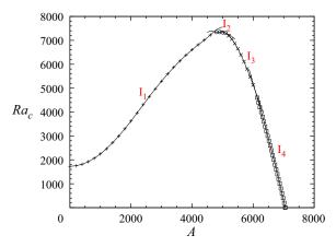
Figure 8. Critical curves for the onset of instability in the Rayleigh–Bénard–Eckart problem in a long 2-D cavity, expressed as  $Ra_c$  as a function of A ( $A_y = 10$ ,  $H_b = 0.338$ , Pr = 1). Four different instabilities (from  $I_1$  to  $I_4$ ) determine the critical curve from the pure Rayleigh–Bénard threshold at  $Ra_0 = 1728.83$  to the pure streaming threshold at  $A_c = 7051.36$ .
