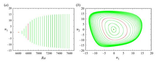
Figure 17. Bifurcation diagram (a) and phase diagram (b) giving the periodic orbits above the oscillatory instability threshold ( $Ra_c = 6609.92$ , red open circle) for A = 4000 in a 2-D cavity with aspect ratio  $A_y = 10$  ( $H_b = 0.338$ , Pr = 1). The cycle presented in figure 16 is given in red.
