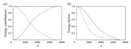
Figure 11. Contributions to the total fluctuating kinetic energy budget  $(E'_s)$  (shear, solid curve),  $E'_b$  (buoyancy, dashed curve)) (a) and energy factors  $R_s$  (connected to shear, solid curve) and  $R_b$  (connected to buoyancy, dashed curve) (b) for the critical perturbations at threshold as a function of the acoustic streaming parameter A (2-D cavity with  $A_v = 10$ ,  $H_b = 0.338$ , Pr = 1).
