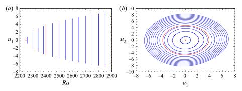
Figure 14. Bifurcation diagram (a) and phase diagram (b) giving the periodic orbits above the oscillatory instability threshold ( $Ra_c = 2246.97$ , red open circle) for A = 1000 in a 2-D cavity with aspect ratio  $A_y = 10$  ( $H_b = 0.338$ , Pr = 1). The cycle presented in figure 13 is given in red.
