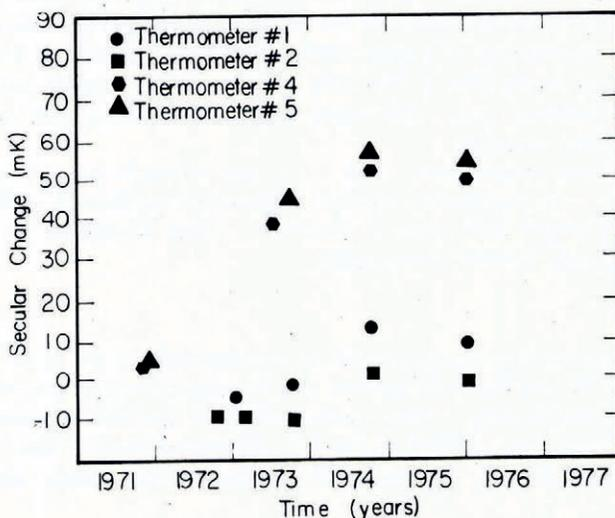
Fig. 1. Secular change versus time for thermometers 1, 2, 4, and 5. The secular change,  $\Delta T = T_0 - T$ , where  $T_0$  is the observed temperature and  $T$  is the calibration temperature.
