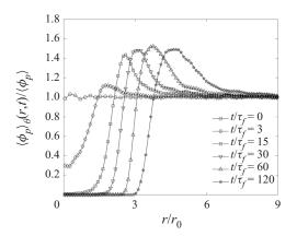
Figure 5. Evolution of the azimuthally averaged volume fraction for a particle-laden Lamb–Oseen vortex with  $St_{\Gamma} = 0.4$ . Owing to their inertia, the particles are progressively expelled from the vortex core, leading to the formation of a ring particle cluster.
