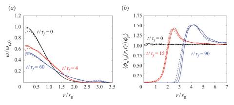
Figure 15. Effect of varying the grid resolution from fine (solid), medium (dash-dotted), to coarse (dashed) in Eulerian–Lagrangian simulations of particle-laden Lamb–Oseen vortex with  $St_{\Gamma} = 0.4$  and Reynolds number  $Re_{\Gamma} = 1700$ . (a) Radial profile of fluid vorticity at  $t/\tau_f = 0$ , 4 and 60. (b) Azimuthally averaged volume fraction distribution at  $t/\tau_f = 0$ , 15 and 30.
