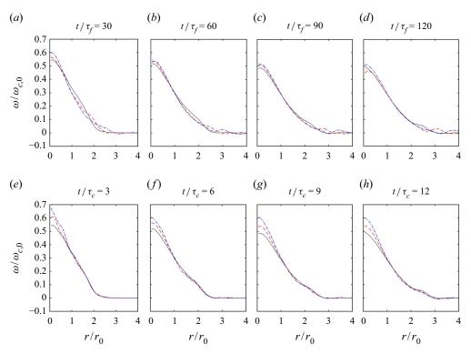
Figure 13. Radial profiles of fluid vorticity normalized by the initial core vorticity for  $St_{\Gamma} = 0.1$  (black solid), 0.2 (red dashed) and 0.4 (blue dash-dotted). (*a*–*d*) Profiles at various  $t/\tau_f$  instants, showing considerable variation of the profile width with Stokes number. (*e*–*h*) Profiles at various  $t/\tau_c$  instants, showing better collapse of the tails of the vorticity distribution across  $St_{\Gamma}$ .
