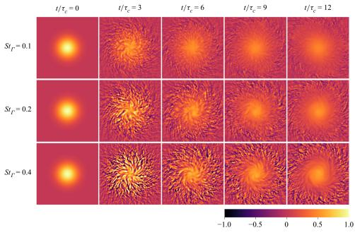
Figure 12. Isocontours of vorticity for the three cases A, B and C (top to bottom) at non-dimensional times  $t/\tau_c = 0, 3, 6, 9$  and 12.
