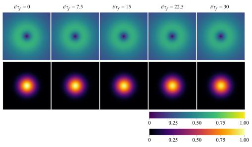
Figure 2. Isocontours of the normalized velocity magnitude  $||u_f||/(\Gamma/2\pi r_0)$  (first row) and axial vorticity  $\omega_z/\omega_{c,0}$  (second row) at successive instants for the single-phase Lamb–Oseen vortex at  $Re_{\Gamma} = 1700$ .
