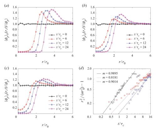
Figure 16. Comparison of the evolution of a particle-laden Lamb–Oseen vortex at  $St_{\Gamma} = 0.4$  and  $Re_{\Gamma} = 1700$  with different initial particle velocities: ( $\bigcirc$ ) matching the fluid velocity at the particle locations; ( $\square$ ) zero velocity; and ( $\Diamond$ ) random velocity. (a–c) Normalized radial profile of volume fraction at successive instants. (d) Vortex core radius. The lines in (d) correspond to power-law fits of the type  $A(t/\tau_f)^m$ .
