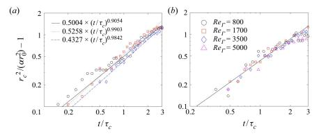
Figure 10. Evolution of the vortex core radius with non-dimensional time  $t/\tau_c$ . (a) Cases A–C:  $Re_{\Gamma} = 17\,000$  and  $St_{\Gamma} = 0.1$  (black  $\bigcirc$ ), 0.2 (red  $\square$ ) and 0.4 (blue  $\diamondsuit$ ). (b) Cases C–F:  $St_{\Gamma} = 0.4$  and  $Re_{\Gamma} = 800-5000$ . The solid line in (b) represents equation (5.5).
