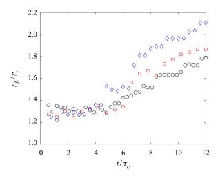
Figure 11. Ratio between void bubble radial location  $r_b$  and fluid core radius  $r_c$  for  $St_{\Gamma} = 0.1$  (black  $\bigcirc$ ), 0.2 (red  $\Box$ ) and 0.4 (blue  $\diamondsuit$ ).
