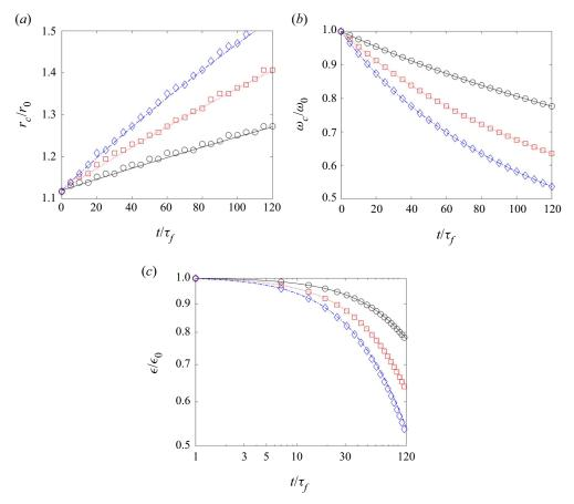
Figure 3. Evolution of the normalized (*a*) vortex core radius, (*b*) centre vorticity and (*c*) enstrophy for an unladen Lamb–Oseen vortex at  $Re_{\Gamma} = 1700$  (black  $\bigcirc$ /solid),  $Re_{\Gamma} = 830$  (red  $\Box$ /dashed) and  $Re_{\Gamma} = 560$  (blue  $\Diamond$ /dash-dotted). Symbols correspond to simulation data. Lines correspond to analytical expressions.
