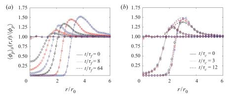
Figure 9. Profiles of azimuthally averaged particle volume fraction for  $St_{\Gamma} = 0.1$  (black  $\bigcirc$ ), 0.2 (red  $\square$ ) and 0.4 (blue  $\Diamond$ ) at (a)  $t/\tau_f = 0$ , 8 and 64, and (b)  $t/\tau_c = 0$ , 3 and 12. The thick dashed lines in (b) represent trajectories of peak volume fraction. The collapse of the profiles in (b) shows that the clustering time scale  $\tau_c$  controls the evolution of the ring cluster.
