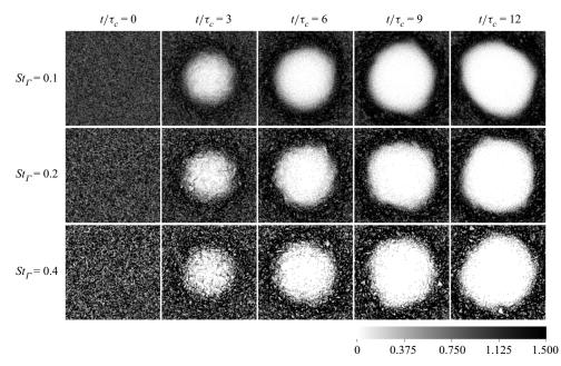
Figure 8. Isocontours of normalized particle volume fraction for three cases A, B and C (top to bottom) at non-dimensional times  $t/\tau_c = 0, 3, 6, 9$  and 12. The similar evolution of the void fraction bubble shows that the clustering time scale  $\tau_c$  controls the large-scale evolution of the particle phase.
