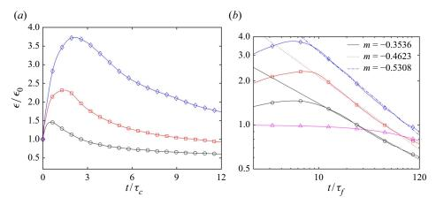
Figure 14. Decaying of the enstrophy at the vortex centre (normalized by its initial value) for various Stokes number. (a) Enstrophy decays for  $St_{\Gamma} = 0.1$  (black  $\bigcirc$ ), 0.2 (red  $\square$ ) and 0.4 (blue  $\diamondsuit$ ) based on time scale  $\tau_f$ . (b) Enstrophy decays with a non-dimensional time based on time scale  $\tau_f$  in log–log scale.
