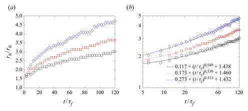
Figure 6. Normalized radius of the void fraction bubble for  $St_{\Gamma} = 0.1$  (black  $\bigcirc$ ), 0.2 (red  $\Box$ ) and 0.4 (blue  $\Diamond$ ). Increasing particle inertia leads to faster formation of a void bubble.
