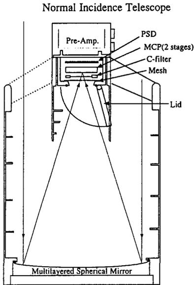
FIGURE 4. Cross section of NIT.
