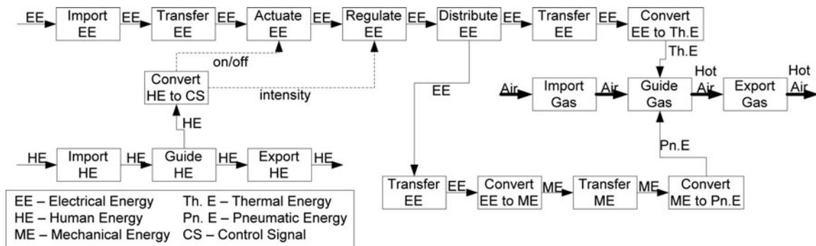
Fig. 3. Function structure of a hairdryer product stored in the Design Repository (<http://repository.designengineeringlab.org/>).
