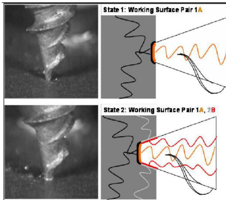
Fig. 6. States of working surface pairs for the contact and channel model for a speed screw (Albers et al., 2008).
