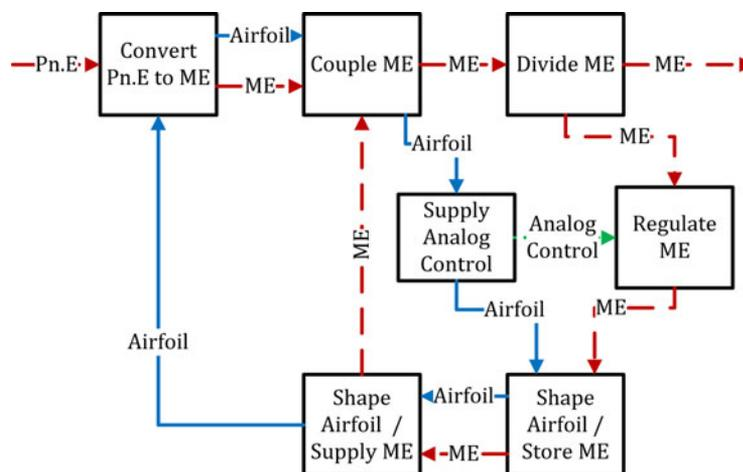
Fig. 7. Function structure for a morphing airfoil (Schultz et al., 2010).
