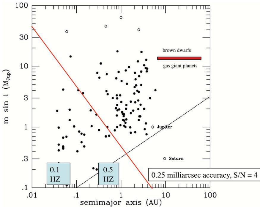
**Figure 2.** CAPSCam astrometric detection limit (red line) for a  $0.1 M_{\odot}$  target star at a distance of 5 pc, assuming astrometric accuracy of 0.25 mas and a signal to noise ratio of 4. Also shown are the approximate radial extents of the habitable zone for target stars with masses of 0.1 and  $0.5 M_{\odot}$ .
