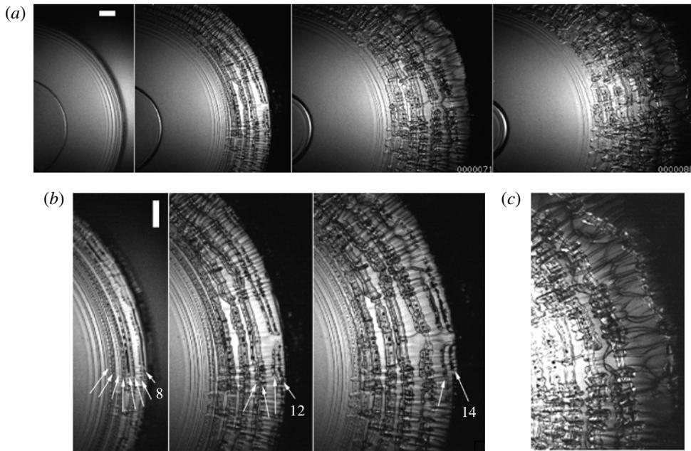
FIGURE 20. Bubble rings and vortex entanglement ( $Re = 12\,900$ ,  $\alpha = 0.80$ ). (a) Frames shown are 8, 22, 41 and 58  $\mu\text{s}$  from first contact on ethanol ( $\delta = 250\ \mu\text{m}$ ). (b) Careful examination of the fine bubbles, shows 14 separate bubble rings, which are pointed out by the arrows. (c) Close-up of the vortex tangles at  $t = 58\ \mu\text{s}$ . The scale bars are 100  $\mu\text{m}$  long. See also supplementary movie.
