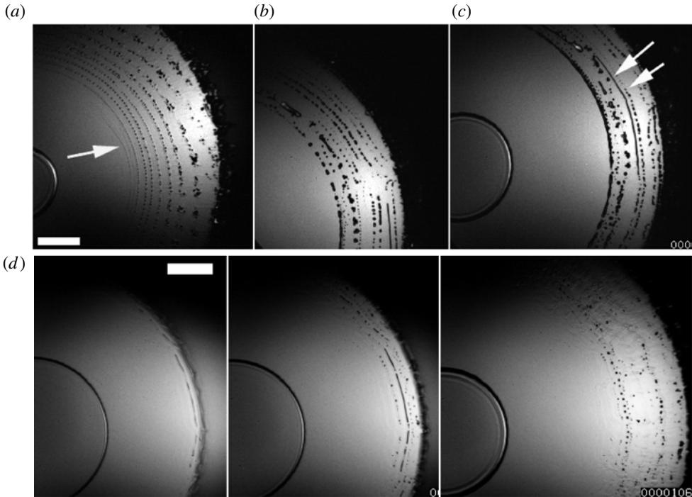
FIGURE 10. Effect of pool depth on the bubble rings for a water drop impacting on methanol, with  $\delta \approx 25$  (a),  $50$  (b) and  $75\ \mu\text{m}$  (c) ( $Re = 12\,900$ ,  $\alpha = 0.80$ ). The frames are all shown  $24\ \mu\text{s}$  after the first contact in (a–c). (d) Deeper methanol pool with  $\delta \approx 500\ \mu\text{m}$ . Frames shown at  $10$ ,  $14$  and  $28\ \mu\text{s}$  after first contact. The scale bars are  $200\ \mu\text{m}$  long. See also supplementary movies.
