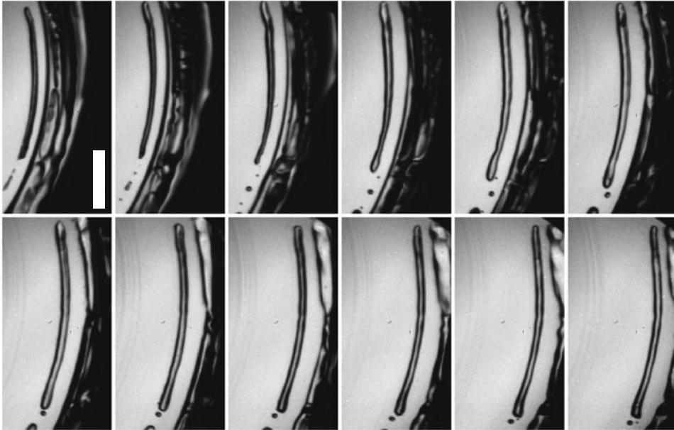
FIGURE 16. Entrapment of a large air cylinder for a water drop impacting on a thin film of methanol ( $Re = 11\,400$ ,  $\alpha = 1.05$ ,  $\delta = 50\ \mu\text{m}$ ). The small bubble at the bottom right of the long cylinder makes a complete rotation around the cylinder between frames 4 and 12. The frames are shown  $4\ \mu\text{s}$  apart. The scale bar is  $200\ \mu\text{m}$  long.
