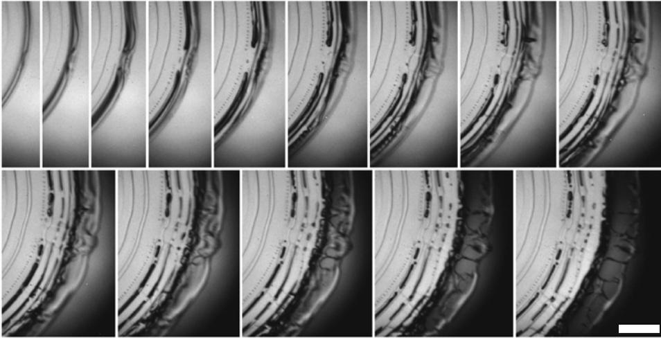
FIGURE 14. Details of the ejecta sheet breakup, for a water drop impacting on a thin film of ethanol ( $Re = 11\,700$ ,  $\alpha = 0.79$ ,  $\delta = 75\ \mu\text{m}$ ). The ejecta sheet starts to puncture in the second frame of the second row. The growth of the holes leaves tendrils connecting the neck to the liquid rim. The scale bar is  $200\ \mu\text{m}$  long. Frames are shown  $2\ \mu\text{s}$  apart.
