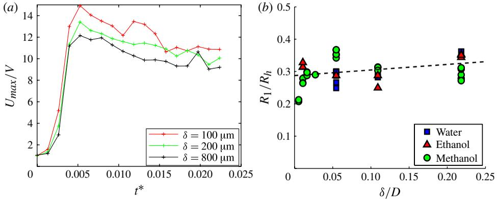
FIGURE 12. (a) Maximum velocity  $U_{max}$  in the liquid from the numerical simulations in figure 11, for three different pool depths. (b) Experimental observation of the first bubble ring entrapment radius ( $Re = 12\,900$ ,  $\alpha = 0.80$ ) for different pool depths.
