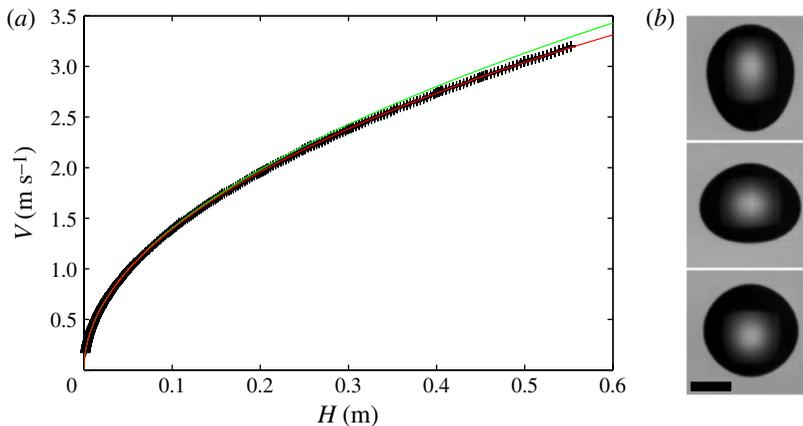
FIGURE 2. (a) Drop velocity  $V$  versus falling height  $H$ . The green line corresponds to  $\sqrt{2gH}$ , while the red line is our fitting equation. (b) Typical drop shapes in air: prolate ( $\alpha > 1$ ,  $H = 31.2$  cm,  $Re = 11\,300$ ), oblate ( $\alpha < 1$ ,  $H = 41.8$  cm,  $Re = 12\,900$ ) and close to spherical ( $\alpha \simeq 1$ ,  $H = 44.5$  cm,  $Re = 13\,300$ ). The scale bar is 2 mm long.
