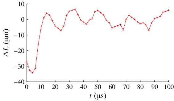
FIGURE 17. (Colour online) Tracking of a  $2\ \mu\text{m}$  particle rotating around a vortex core for a drop impacting on a pool of ethanol ( $Re = 11\,400$ ,  $\alpha = 1.05$ ,  $\delta = 125\ \mu\text{m}$ ).  $\Delta L$  is the distance from the initial position, minus the mean radial translation component identified by a linear regression. The period of rotation is here  $\sim 18\ \mu\text{s}$ .
