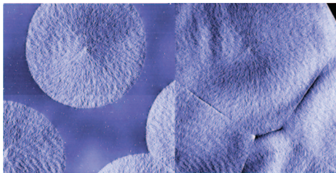
Figure 4: Two high-resolution 20 \times 20 \mu\text{m} AFM scan frames show PHBV crystal growth from amorphous phase after quenching. The image on the left shows one AFM image frame of spherulite growth. The image on the right shows a single AFM image frame of the dominant lamellae slowing their growth to a stop. Each of these 13-megapixel images was captured in minutes, enabling researchers to further explore the sample's micro- and nano-scale features offline.
