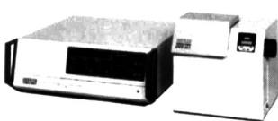
• **The easy-to-operate PIT Series thermal constants analyzers** utilize the AC calorimetric method to determine thermal diffusivity, specific heat, and thermal conductivity from RT to 500°C on specimens less than 0.3 mm thick. Measurement possible in any direction in the specimen surface. Cryogenic option available.
