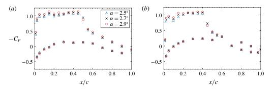
FIGURE 5. Static pressure distributions at two outboard spanwise stations around structural buffeting onset at three angles of attack and M = 0.80: (a)  $\eta = 0.73$  and (b)  $\eta = 0.93$ .
