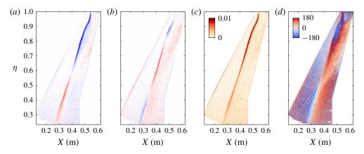
FIGURE 24. DMD mode at 83 Hz: (a) real part, (b) imaginary part, (c) magnitude and (d) phase angle in degrees. The spatial amplitudes in (a) and (b) are coloured from blue to red, representing opposite signs (-0.01 to 0.01).
