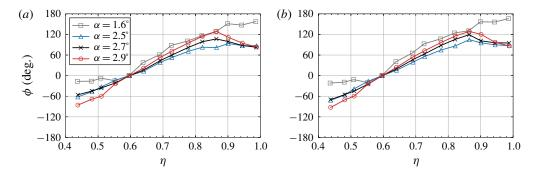
FIGURE 18. Phase angle variation along shock at selected frequencies of low-frequency shock unsteadiness at pre- and post-onset conditions at M=0.80: (a) 72 Hz and (b) 80 Hz.
