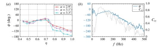
FIGURE 22. Phase angle variation along shock representing higher-frequency outboard-running oscillations at M=0.80: (a) phase angle with span at 216 Hz and (b) phase angle (solid line) and coherence levels (dotted line) with frequency for two points along shock, between  $\eta=0.87$  and  $\eta=0.99$ , at  $\alpha=3.3^\circ$ . Dashed blue line in (b) indicates linear fit between 200 and 400 Hz.
