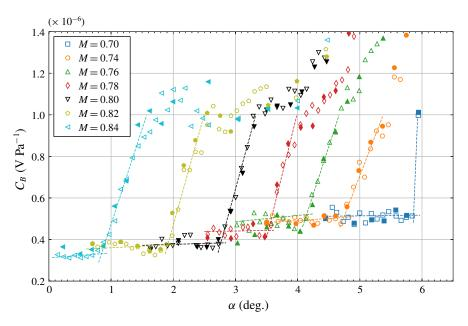
FIGURE 3. Dimensional buffeting coefficient over angle of attack for a range of Mach numbers: open symbols represent fine-pitch runs with DDAS, filled symbols denote coarser-pitch runs that also include DPSP acquisition.
