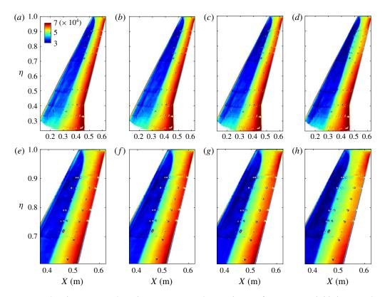
FIGURE 4. Time-averaged static pressure on the suction surface at M=0.80 in Pascal: (a)  $\alpha=2.5^{\circ}$ , (b)  $\alpha_b=2.7^{\circ}$ , (c)  $\alpha=2.9^{\circ}$ , (d)  $\alpha=3.3^{\circ}$  and (e-h) show the magnified outboard section corresponding to (a-d), respectively.
