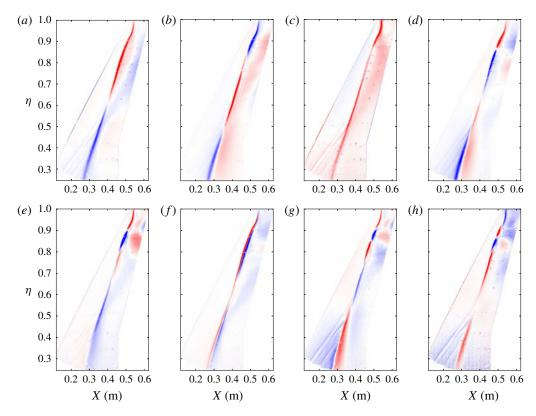
FIGURE 14. Spatial component of dominant POD modes at M=0.80 and  $\alpha=3.3^{\circ}$  capturing low-frequency shock unsteadiness and shock buffet. The spatial amplitudes are coloured from blue to red, representing opposite signs (-0.01 to 0.01); modes 1, 3, 4, 7, 8, 9, 11 and 13 are denoted by (a-h). Structure-dominated modes are not shown.
