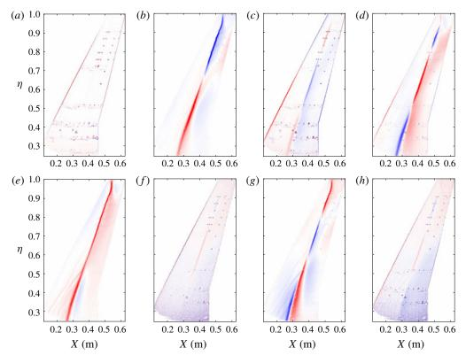
FIGURE 11. Spatial component of first eight POD modes at M = 0.80 and  $\alpha = 2.9^{\circ}$ . The spatial amplitudes are coloured from blue to red, representing opposite signs (-0.01 to 0.01); modes 1 to 8 are denoted by (a-h).
