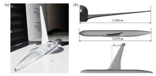
FIGURE 1. RBC12 half-model: (a) installation on wind tunnel floor and (b) geometrical information (semi-span of 1.104 m includes the model plinth of 0.019 m).
