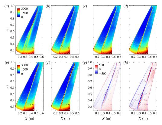
FIGURE 9. Standard deviation of DPSP static pressure in Pascal at M=0.80: (a)  $\alpha=1.6^{\circ}$ , (b)  $\alpha=2.5^{\circ}$ , (c)  $\alpha_b=2.7^{\circ}$ , (d)  $\alpha=2.9^{\circ}$ , (e)  $\alpha=3.1^{\circ}$  and (f)  $\alpha=3.3^{\circ}$ . Relative standard deviation between pairs of  $\alpha$ : (g)  $\sigma_{\alpha_b=2.7^{\circ}}-\sigma_{\alpha=2.5^{\circ}}$  and (h)  $\sigma_{\alpha=2.9^{\circ}}-\sigma_{\alpha_b=2.7^{\circ}}$ .
