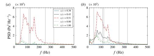
FIGURE 6. Chordwise PSD data at  $\eta=0.80$  for two angles of attack around structural buffeting onset at M=0.80: (a)  $\alpha_b=2.7^\circ$  and (b)  $\alpha=2.9^\circ$ . The vertical lines denote the structural frequencies of the model.
