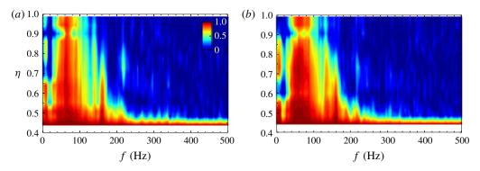
FIGURE 17. Magnitude-squared coherence levels of pressure signals along shock for two angles of attack beyond structural buffeting onset at M = 0.80: (a)  $\alpha = 2.9^{\circ}$ , (b)  $\alpha = 3.3^{\circ}$ .
