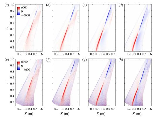
FIGURE 13. Instantaneous snapshots at M = 0.80 and  $\alpha = 2.9^{\circ}$ , starting from t = 0.0175 s in steps of  $\Delta t = 0.0015$  s, coloured by static pressure deviation from mean, in Pascal: (a-d) POD reconstructed snapshots using modes 2, 4 and 5 and (e-h) original snapshots.
