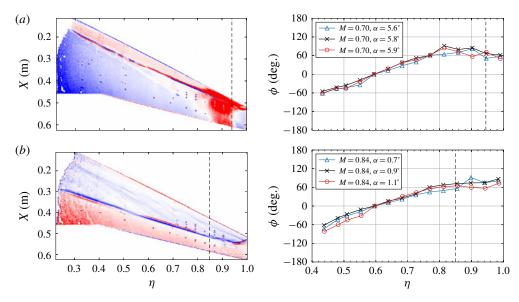
FIGURE 20. Relative standard deviation around structural buffeting onset and phase angle variation computed at 80 Hz along shock at: (a) M = 0.70,  $\sigma_{\alpha=5.9^{\circ}} - \sigma_{\alpha_b=5.8^{\circ}}$  and (b) M = 0.84,  $\sigma_{\alpha=1.1^{\circ}} - \sigma_{\alpha=0.7^{\circ}}$ . The same symbol key of figure 19 is used.
