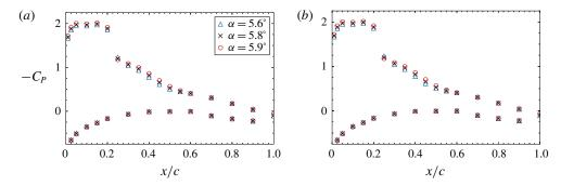
FIGURE 21. Static pressure distributions at two outboard spanwise stations around structural buffeting onset at M = 0.70: (a)  $\eta = 0.73$ , (b)  $\eta = 0.93$ .
