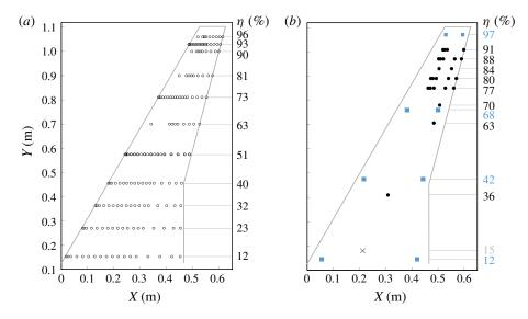
FIGURE 2. Locations of instrumentation on wing's upper surface: (a) 162 static pressure taps and (b) unsteady pressure transducers, accelerometers and a root strain gauge denoted by the black filled circles, blue filled squares, and the grey cross, respectively.
