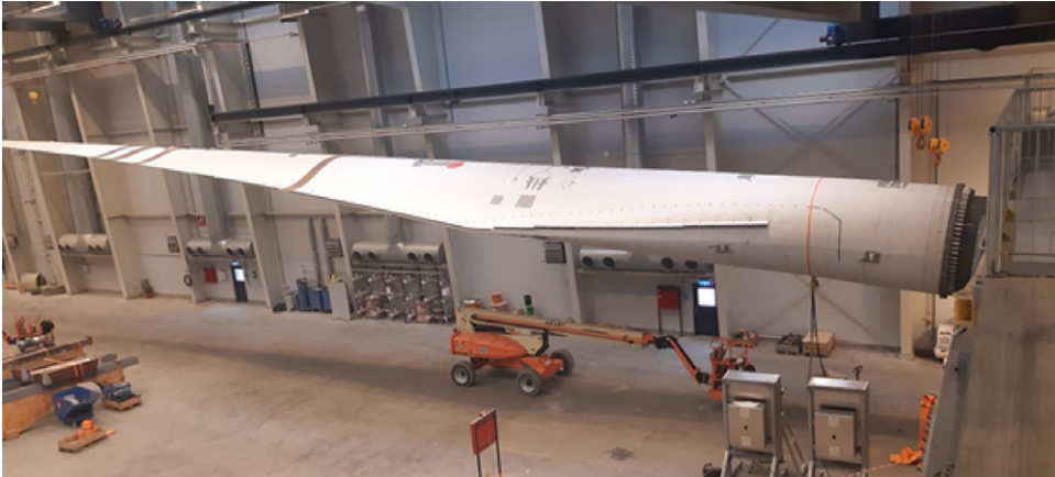
Figure 1. A 52-meter blade on test stand at the Siemens Gamesa Blade Test Center in Aalborg, Denmark. The blade is mounted pressure side up for flapwise fatigue testing. The image shows the blade without the fatigue exciter mounted.
