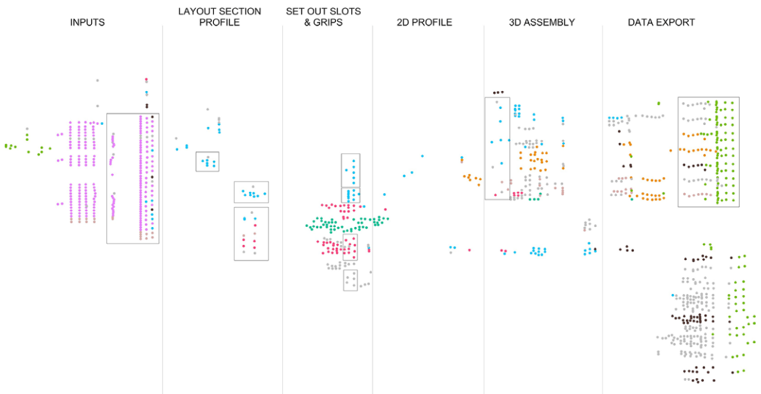
Figure 14. Groups of design components (rectangles) and design phases (labels) as set by the Wren developer to order 1086 design components, compared with the modules (colour) as recognised by the modularity algorithm in Figure 12. 20
