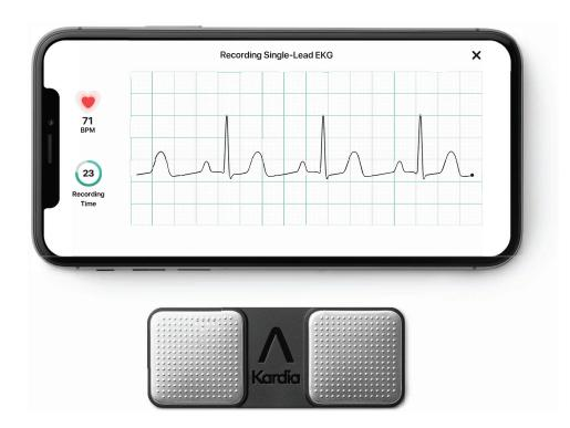
**Figure 1.** The KardiaMobile single-lead ECG device. Photograph by AliveCor, Mountain View, CA
