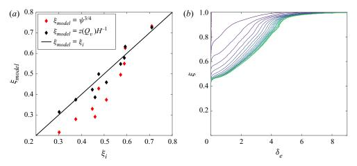
FIGURE 11. (a) Comparison of the predicted steady-state interface heights for the two models considered in the text with the measured interface height from the experiments. (b) An example of the evolution of the ambient buoyancy profile, taken from experiment 5, as it tends to a steady state.
