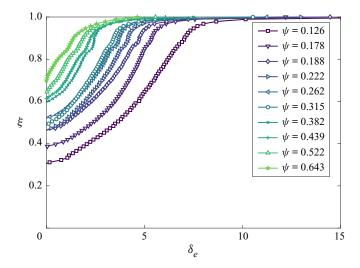
FIGURE 12. Steady-state ambient buoyancy profiles of the ventilated experiments. The data points shown are sub-sampled at a resolution of  $\Delta \xi = 0.011$  to aid clarity to the figure. This corresponds to the resolution at a height of  $\xi = 0.90$ .
