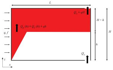
FIGURE 2. Schematic of the ventilated distributed wall-source plume with a finite source volume flux, where the box is connected to the exterior environment by an open vent at the bottom of the box and a gear pump (not shown) is forcing ventilation by extraction of fluid through openings at the top.
