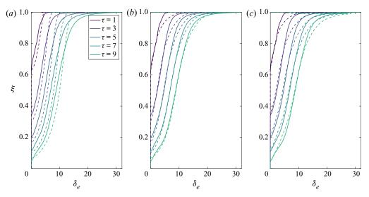
FIGURE 10. Comparison of the filling box peeling models (dashed curves) compared with experiment 1 (solid curves) for non-dimensional times  $\tau = 1, 3, 5, 7$  and 9 for (*a*) FBM (i), (*b*) FBM (ii) and (*c*) FBM (iii) discussed in the text.
