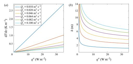
FIGURE 16. The (a) ambient temperature gradient and (b) steady-state interface height as functions of the heat flux for selected ventilation flow rates in a typical atrium.
