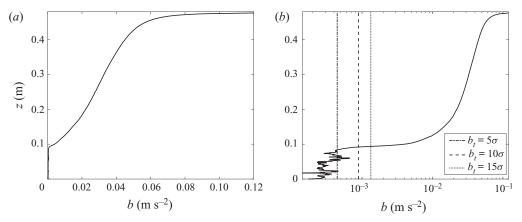
FIGURE 6. (a) Ambient buoyancy profile of the filling box experiment. (b) The same data presented with a logarithmic buoyancy scale. The vertical dashed line shows the threshold  $b = b_t = 10\sigma$  used to identify the first front interface, where  $\sigma$  is the standard deviation of the ambient buoyancy from an undyed background image. The other two lines show  $b = 0.5b_t$  and  $b = 1.5b_t$ .
