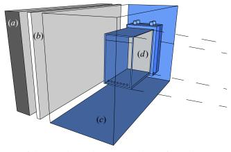
FIGURE 4. Diagram of the experimental set-up used to perform dye attenuation of the filling box and ventilated experiments showing the (a) LED light bank, (b) light diffuser, (c) large reservoir tank and (d) apparatus illustrated in figure 3. The dashed lines indicate the measuring window of the camera which is placed 10 m from the edge of the large reservoir to minimise the parallax error.
