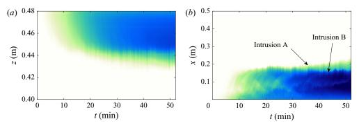
FIGURE 14. (a) Horizontally and (b) vertically spatial-averaged evolution of the blue dye added to the source solution. The regions used to spatial average are shown in figure 13(c). The figures suggest that there is no net vertical motion within the stratified ambient region 0.20 m < x < 0.50 m,  $h_i < z < 0.42$  m.
