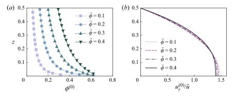
Figure 4. (a) Local particle concentration profile  $\phi^{(0)}$  and (b) the normalised velocity profile,  $u_r^{(0)}/\bar{u}$ , as a function of z for varying depth-averaged concentrations  $\bar{\phi}$ .
