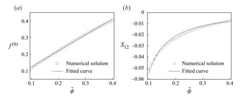
Figure 6. (a) The numerical solution of the leading order flux,  $f^{(0)}$ , is plotted as a function of depth-averaged concentration  $\bar{\phi}$ . The solid line indicates the linear fit. (b) The solution of  $S_{12}$  is plotted for varying depth-averaged concentration,  $\bar{\phi}$ , and is fitted with a function  $-0.0022 \times \phi^{-1.399}$ .
