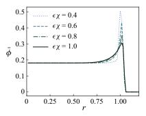
Figure 8. The numerical solution of depth-averaged particle concentration,  $\bar{\phi}_{up}$ , as function of r is plotted for various values of  $\epsilon \chi$  at t = 14 s and  $\phi_0 = 0.2$ . As  $\epsilon \chi$  increases, the increase in  $\bar{\phi}_{up}$  becomes less steep.
