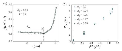
Figure 3. (a) Particle flux, f, plotted as a function of r when  $\phi_0 = 0.25$ . Here,  $R_{in}(t)$  is defined at the location that f starts increasing from a constant value upstream. In (b),  $R_{in}(t)$  increases linearly with  $t^{1/2}$  for varying  $\phi_0$
