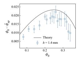
Figure 7. The difference between the initial concentration and the depth-averaged particle concentration,  $\phi_0 - \bar{\phi}_{up}$ , in Region II is plotted as a function of  $\phi_0$ . The solid line represents the numerical solution from the simplified suspension balance model with the constraint of the particle volume conservation. The square markers indicate the experimental data for h = 1.4 mm.
