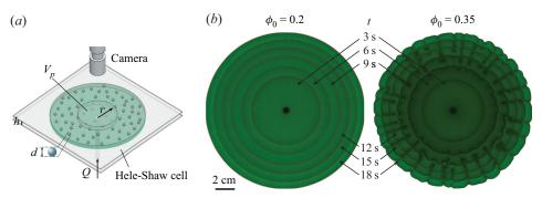
Figure 1. (a) A schematic of the experimental set-up. (b) Time-elapsed images of the suspension injected into a Hele-Shaw cell with gap thickness h = 1.4 mm, at  $\phi_0 = 0.2$  (a) and  $\phi_0 = 0.3$  (b). Here, the particle diameter d and the injection flow rate Q correspond to  $d = 125 \,\mu\text{m}$  and  $Q = 150 \,\text{ml} \,\text{min}^{-1}$ , respectively.
