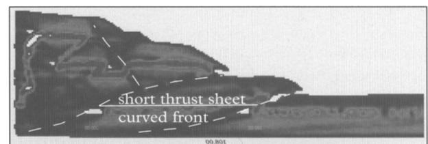
CT scan of sandbox model with high basal friction.
