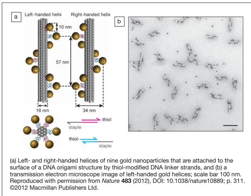
predicted theoretically, coupling of plasmon waves along the helices results in increased absorption of specific polarizations of light, and left- and right-handed helices show a mirror-image peak/dip close to the surface plasmon resonance frequency at 524 nm.
