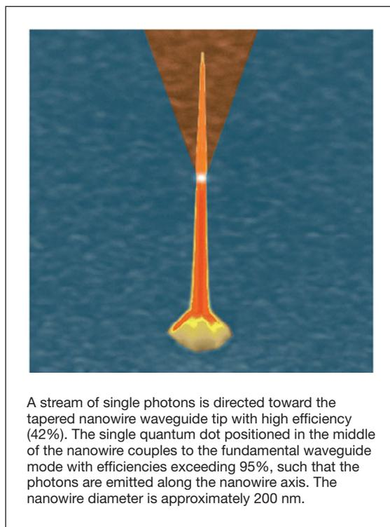
A stream of single photons is directed toward the tapered nanowire waveguide tip with high efficiency (42%). The single quantum dot positioned in the middle of the nanowire couples to the fundamental waveguide mode with efficiencies exceeding 95%, such that the photons are emitted along the nanowire axis. The nanowire diameter is approximately 200 nm.
