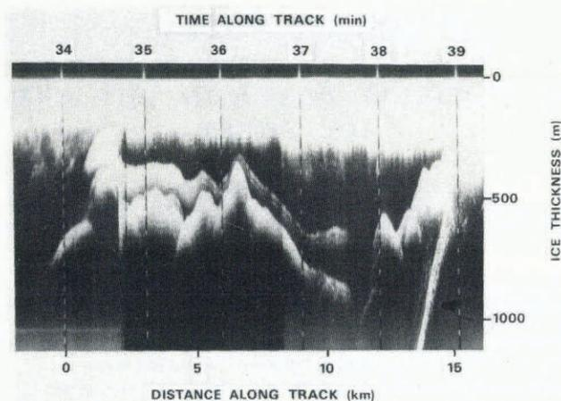
Fig. 1. Print of radio echo record showing a strong reflecting layer within the ice but at some distance above bedrock. (Note that the ice-thickness scale refers to times after 34.7 min, where there is a change of vertical scale.)
