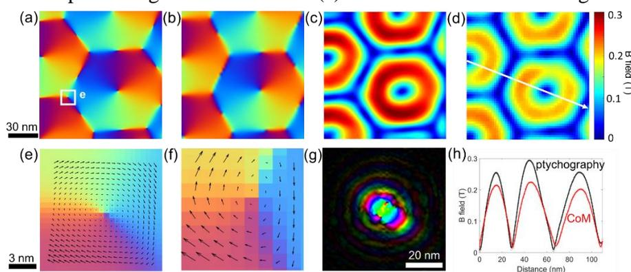
**Figure 2.** Comparison of magnetic induction field determined from ptychography and direct center of mass (CoM). (a) & (c) Field direction and magnitude from ptychography; (b) & (d) Field direction and magnitude from CoM; (e) & (f) Field vectors (selected regions marked on (a)) determined from ptychography (e) and CoM (f); (g) Electron probe retrieved via ptychography; (h) Line profiles of field magnitude from ptychography (black) and CoM (red) (profile of white line in (d)).
