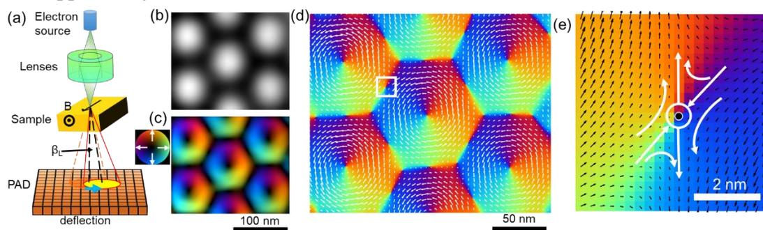
**Figure 1.** Magnetic induction field measured via Lorentz electron ptychography. (a) Lorentz STEM setup. (b) Phase shift reconstructed via Lorentz electron ptychography for skyrmion lattice in single crystal FeGe at 94 K. (c) Magnetic induction field vector calculated from the phase shift. (d) Magnetic induction field direction with arrows representing the field vectors. (e) An anti-vortex from the region marked on (d).
