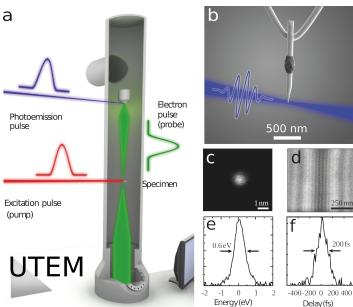
**Figure 1.** (a) Schematic of Göttingen UTEM, with stroboscopic laser pump and electron probe principle. (b) Photoelectron pulses are generated by illumination of a heated tungsten tip emitter with a ZrO2 reservoir. (c) Minimum electron spot size. (d) Photoelectron hologram measured with a biprism (adapted from [8]). (e,f) Measured optimal spectral and temporal width.
