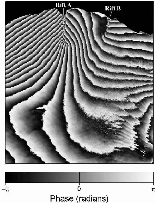
Fig. 6. Interferogram derived from ERS-1 orbit 24526 (24 March 1996) and ERS-2 orbit 04309 (25 March 1996) of the eastern part of the AIS front. The topographic contribution to the phase has been removed using topography provided by a digital elevation model derived from ERS-1 satellite radar altimetry (Fricker and others, 2000a).
