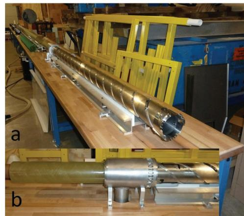
**Fig. 11.** (a) Core-processing line. (b) FED assembly with fiberglass netting deployment sleeve.
