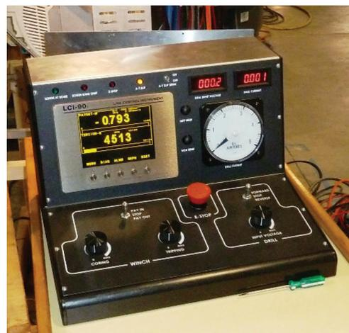
Fig. 10. Drill control console.
