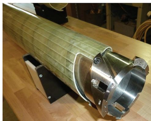
Fig. 8. Fiberglass outer tube with dry core barrel and cutter head.
