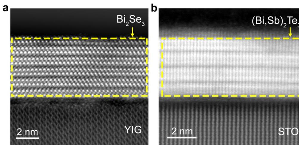
**Figure 2:** (a) Atomic resolution image of a thin Bi<sub>2</sub>Se<sub>3</sub> layer grown on yttrium iron garnet (YIG). The 2D material is used to induce spin-charge conversion in a spintronic device, as discussed in [4]. (b) Atomic resolution image of a thin (Bi,Sb)<sub>2</sub>Te<sub>3</sub> layer grown on strontium titanate (STO). (Bi,Sb)<sub>2</sub>Te<sub>3</sub> is used as a spin channel below an Al<sub>2</sub>O<sub>3</sub>/Py magnetic tunnel junction, as discussed in [5].
