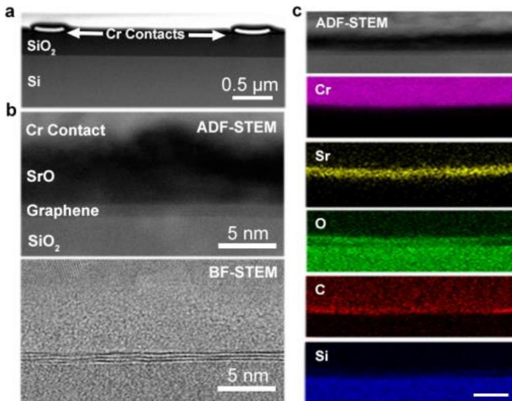
**Figure 1:** (a) Low-magnification image of a graphene spin valve device. The graphene interface is between the SiO<sub>2</sub> layer and Cr contacts. (b) High-magnification ADF-STEM and BF-STEM images showing a 4-layer graphene interface. (c) Energy dispersive X-ray spectroscopy (EDX) elemental maps acquired along the interface; scale bar is 5 nm.
