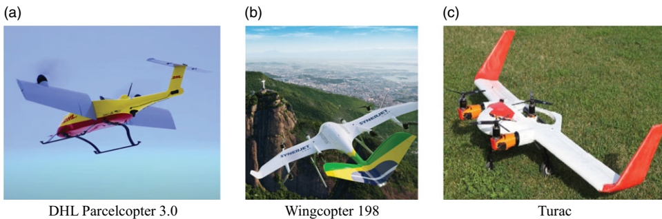
Figure 2. Examples of convertiplane drones.
