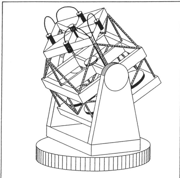
Figure 1 – A possible compact CAT design with four mirrors, each 1.2 metres diameter and feeding fibres at its prime focus
