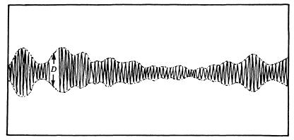
Fig. 2. Section of record showing how the probability distribution P(D) is derived from measurements of the amplitude (D) of the envelope of the interference pattern.
