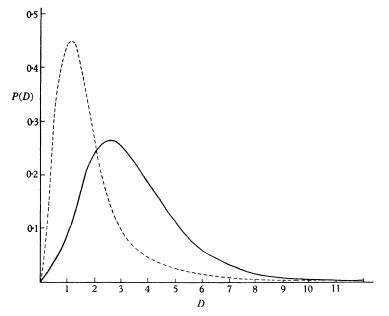
Fig. 3. The probability distribution P(D) of the amplitude of the record D. The full curve represents the observations whilst the theoretical curve for a uniform spatial distribution of sources is shown dotted.
