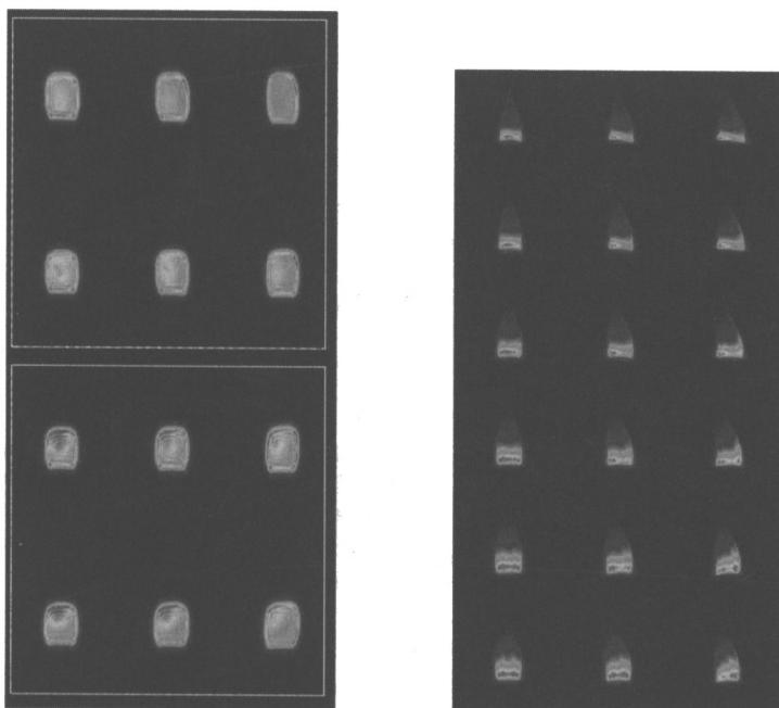
Figure 2. In the left figure are shown the images of the PSF at different locations in the seismology focal plane, demonstrating the optical properties of the instrument. The right figure shows the same thing in the exoplanet focal plane. As there is a bi-prism added in the exoplanet channel, each image of a star is a small spectrum. The dispersion of the bi-prism is along the vertical axis, with the blue part above and the red part below each of the individual spectra.
