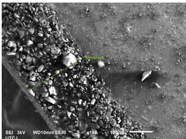
Figure 1. SEM image of transversal section of hydrogel enriched with allantoin.
