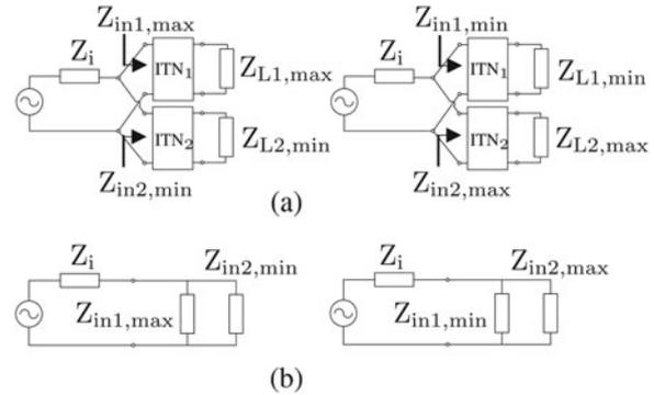
**Fig. 7.** The scheme of the power divider network (PDN). (a) An illustration of the PDN comprising two impedance transformation networks (ITN) in parallel with its two scenarios. (b) The equivalent circuit of the PDN with its two scenarios.
