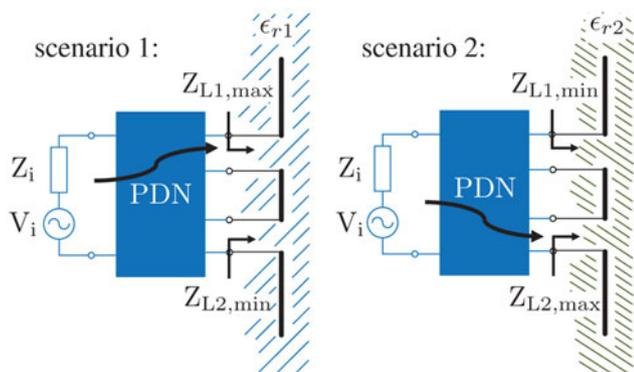
**Fig. 1.** Concept of matching a dual-fed antenna to a source by a power divider network (PDN). Varying antenna feed impedances due to environmental (near-field) changes to the antenna cause the power flow to change from connecting feed one with the source in the first scenario, while connecting feed two with the source in the second scenario.
