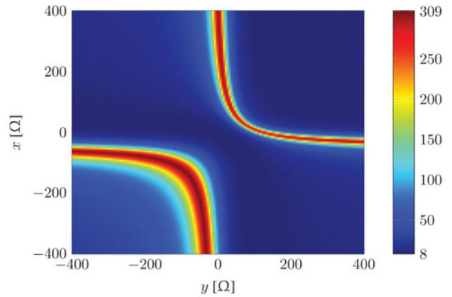
**Fig. 5.** Colormap of  $Re\{Z_{in}|_{Z_i=Z_{i,\min}}\}$  over  $x$  and  $y$  (see (3)) with  $Z_{L,\min} = 20 + j10 [\Omega]$  and  $Z_{L,\max} = 70 - j50 [\Omega]$  arbitrarily chosen. This map is calculated with (3). Dark red indicates the maximum value while dark blue gives the minimum value in ohm. It should be noted that for  $Z_{in}|_{Z_i=Z_{i,\max}}$  (2) is fulfilled for all values of  $x$  and  $y$ .
