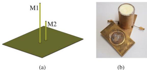
**Fig. 8.** (a) Two monopoles of different length next to each other forming the dual-fed adaptive antenna. (b) Photo of the butter-filled cylindrical resonator (opened for clarity) for determination of the material properties of butter.
