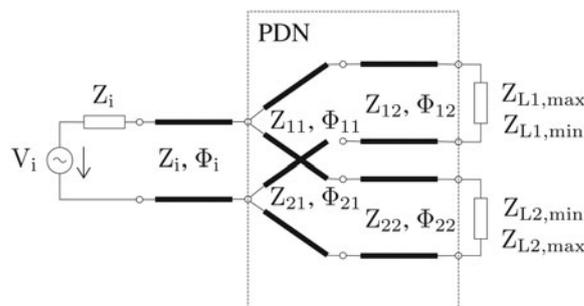
**Fig. 10.** Equivalent circuit of the PDN.
