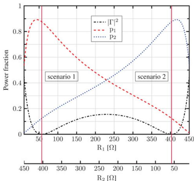
**Fig. 3.** Portions of the maximum power, which the source can deliver: reflected power  $|\Gamma|^2$  (black dash-dotted line), the power dissipated in  $R_1$  ( $p_1$  red dashed line) and the power dissipated in  $R_2$  ( $p_2$  blue dotted line).
