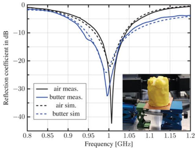
**Fig. 14.** Measured and simulated reflection coefficient of the adaptive antenna for both scenarios (air and butter). The inset picture shows the measurement setup for the scenario with butter.
