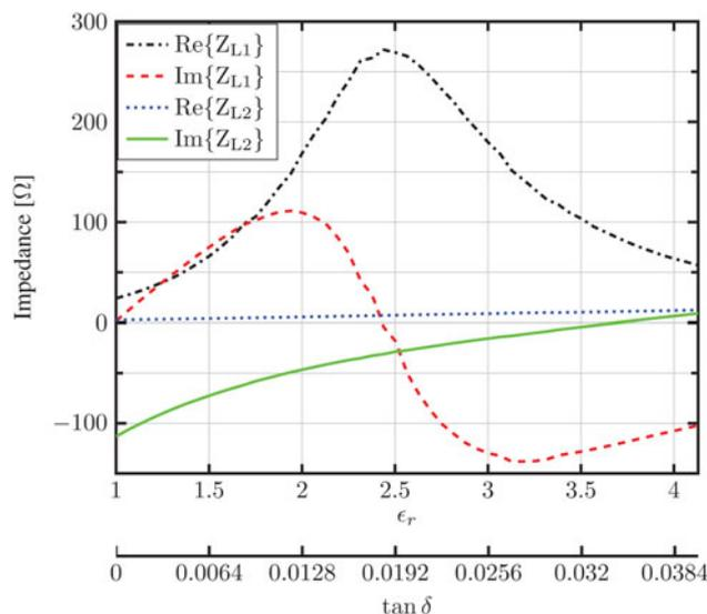
**Fig. 9.** Simulated input impedance of the two monopoles when assuming a linear transition of the relative permittivity and loss tangent from the scenario with air to the one with butter. It holds  $Z_{L1}(\epsilon_r=1, \tan\delta=0) = Z_{L1,max}$ ,  $Z_{L2}(1, 0) = Z_{L1,min}$ ,  $Z_{L1}(4.13, 0.04) = Z_{L1,min}$ , and  $Z_{L2}(4.13, 0.04) = Z_{L2,max}$ .
