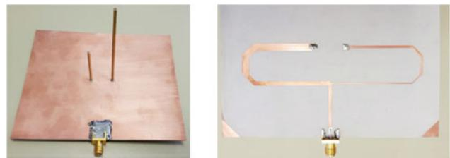
**Fig. 13.** Adaptive antenna prototype. Left: two monopoles over board ground. Right: microstrip PDN and feed.
