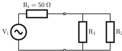
**Fig. 2.** Two resistors in parallel.
