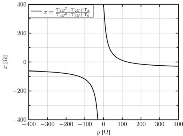
**Fig. 6.** Plotted function of (5) for  $Z_{L,\min} = 20 + j10$  [Ω] and  $Z_{L,\max} = 70 - j50$  [Ω]. This curve gives the relation between  $x$  and  $y$  to obtain the highest possible value of the real part of  $Z_{in}|_{Z_L=Z_{L,\min}}$ . At the same time (2) for  $Z_{in}|_{Z_L=Z_{L,\max}}$  is fulfilled. This curve can be recognized as the maxima of the colormap in Fig. 5.
