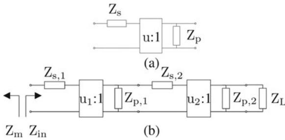
**Fig. 4.** Lumped-element equivalent circuit model. (a) Circuit model of a transmission line. (b) Circuit model of a two-step transmission line-based impedance transformer.
