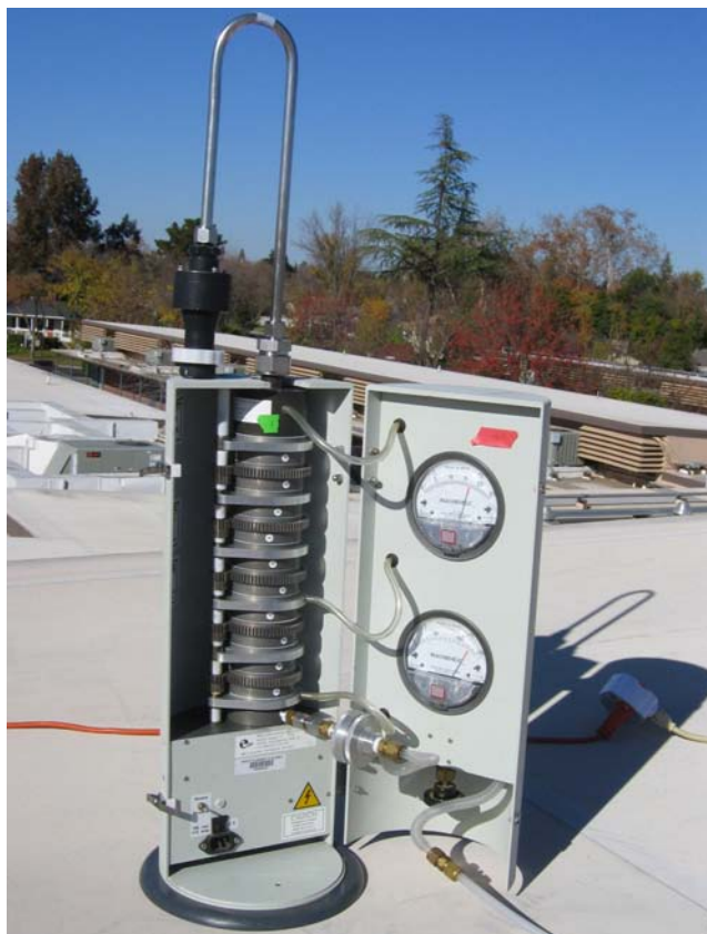
Figure 1 MOUDI sampler atop school gymnasium during sample collection
