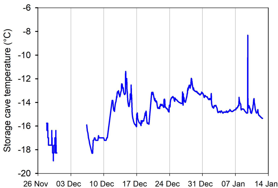
Fig. 9. Skytrain ice rise ice core storage cave temperature. Generally, the storage cave remained below -12^{\circ}\text{C} through most of the season. The temperature spike in January was a brief period of 1 h when the storage cave was opened for moving out ice core boxes to the aircraft for uplift from the field site.
