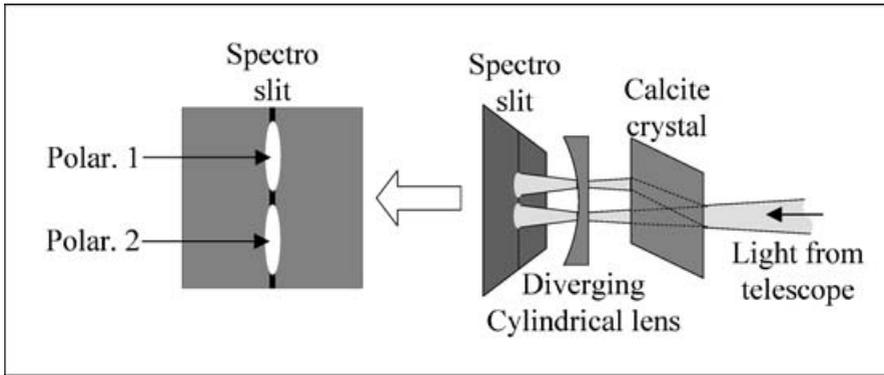
**Figure 4.** The additional optics to split polarizations and spread the focal spots along the spectrograph slit. A calcite crystal ( $CaCO_3$ ) transforms the convergent beam from the telescope into two convergent beams, one with polarization 1, the other with polarization 2. The cylindrical diverging lens spreads the two spots in the direction of the spectrograph slit.
