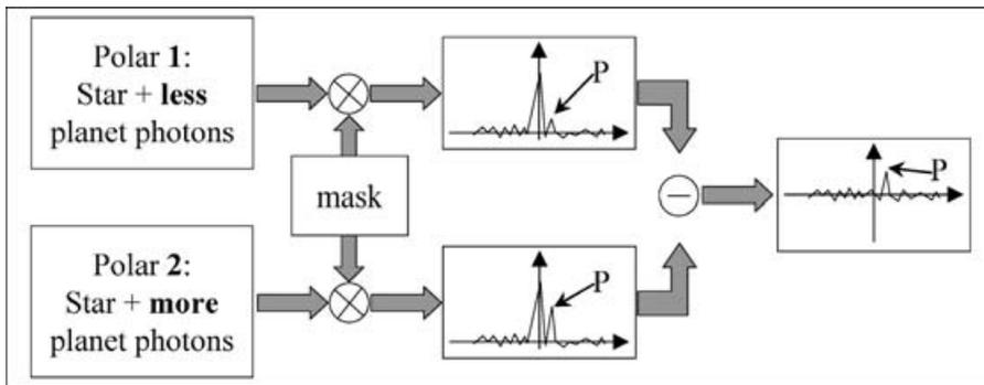
**Figure 3.** How the planetary signal should appear. The spectra in two complementary polarization states are convoluted with the same Dirac mask. Both correlation functions are dominated by the stellar photons (small Doppler shift). The small planetary Doppler shifted pike is present with different amplitude in both signals. When subtracting one to the other, the stellar features should cancel, and the planetary signature should remain, hopefully emerging out of the residual noise.
