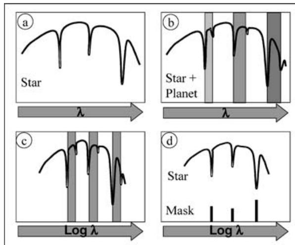
**Figure 2.** The sketched spectrum of a star and a Pegaside. (a) The spectrum of the star alone. (b) The spectrum of the star + planet Doppler-shifted. (c) The same in  $\log(\lambda)$  coordinate, so as to make the Doppler shift constant. (d) The spectrum of the star and the correlation Dirac mask.
