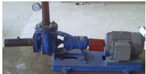
Fig. 2. Centrifugal pump of POVAL, type NVA 150-5 [8].
